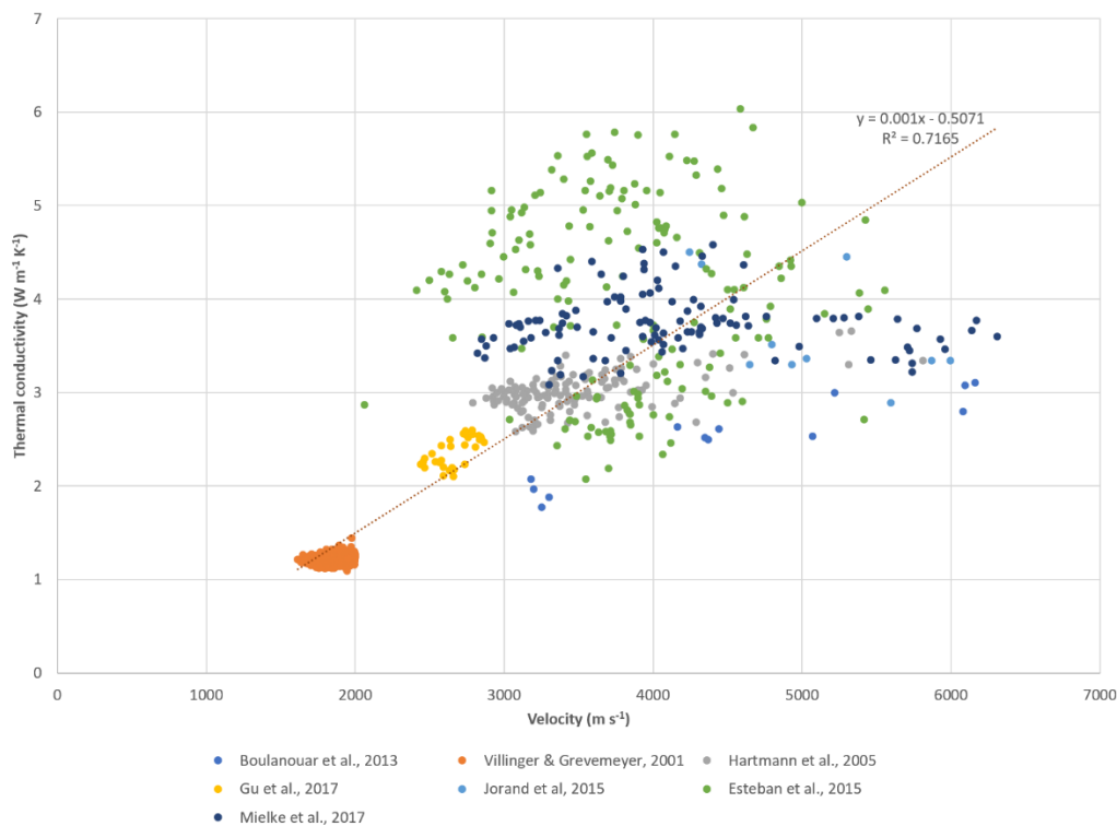
Figure 5: Empirical velocity to thermal conductivity transform utilising experimental datasets from published literature. These measurements are made on samples in laboratory conditions and represent a wide range of lithologies. Furthermore, only results from wet sample measurements are displayed, as the transform will be applied in the shallow subsurface where there is very likely to be fluid fill (for example the GHSZ). Measurements were made using transient method (using optical scanning equipment). GHSZ = Gas hydrate stability zone.
