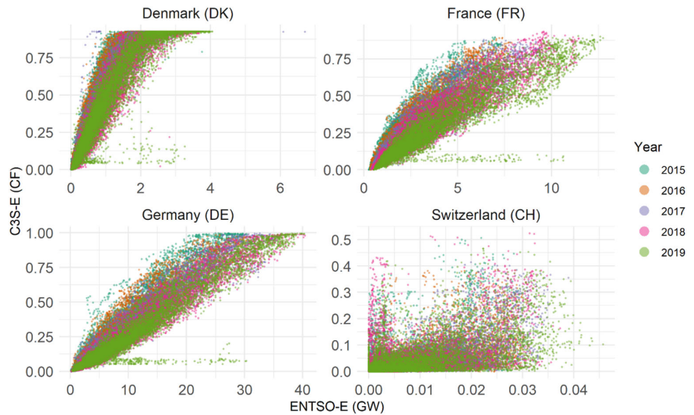
FIGURE 11 Scatter plot for onshore wind in four selected countries. The C3S-E capacity factor is represented against ENTSO-E TP actual generation. Dots' colour correspond to different years.
