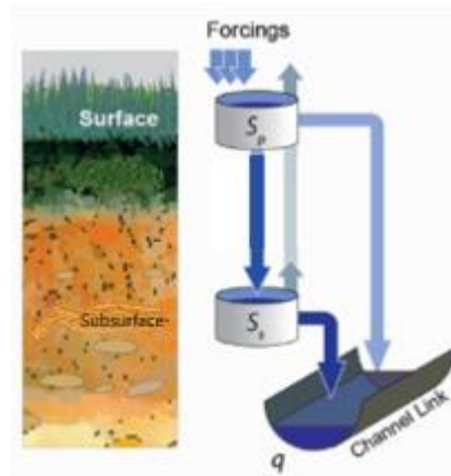
Figure 5 Mathematic and pictorial description of the constant runoff model implemented in HLM-Web.
