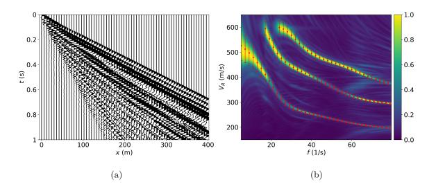
Figure 1: Synthetic seismogram (a) and its V-f spectra with the confidence intervals of picking shown in red color (b) for PGV-model.
