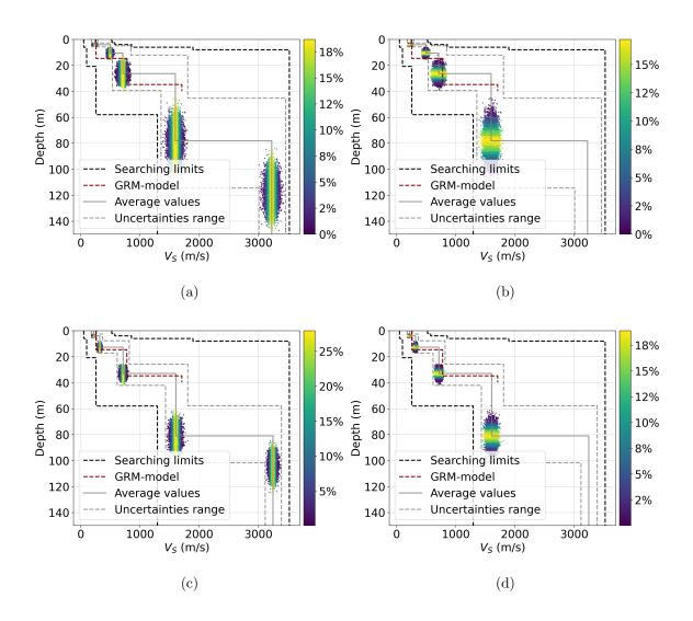
Figure 12: Results of uncertainty quantification while field data processing: S-wave errors distributions (a) and thickness errors distributions (b) by uni-mode inversion and S-wave errors distributions (c) and thickness errors distributions (d) by multimode inversion. Color scaling means the percentage of hit rate in pixel.
