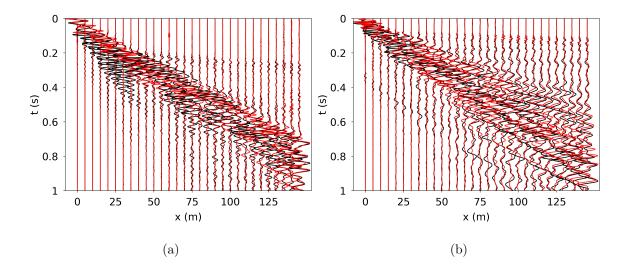
Figure 10: Field seismogram (y-y) of horizontal velocity displacement with using corresponding horizontal source for waves generation (a) and field seismogram (z-z) of vertical velocity displacement with using corresponding vertical source (b). Seismograms for source 0 m (first point of the seismic profile) and source 145 m (end point of the seismic profile) are shown in black and red colors, respectively
