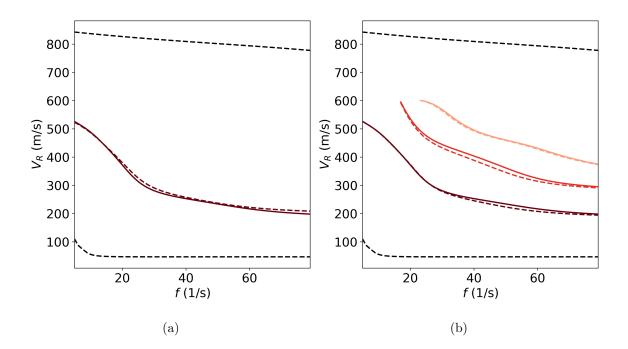
Figure 5: The comparison of the phase velocity dispersion curves computed by average values of uni-mode (a) multi-mode (b) inversion for PGV-model. The true and restored dispersion curves are shown by solid and dotted colored lines correspondingly, the searching limits are shown by black dotted lines.
