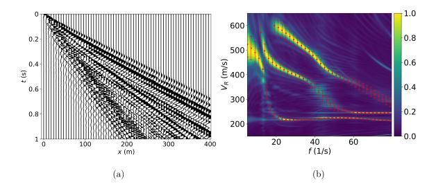
Figure 6: Synthetic seismogram (a) and its V-f spectra with the confidence intervals of picking shown in red color (b) for LVL-model.
