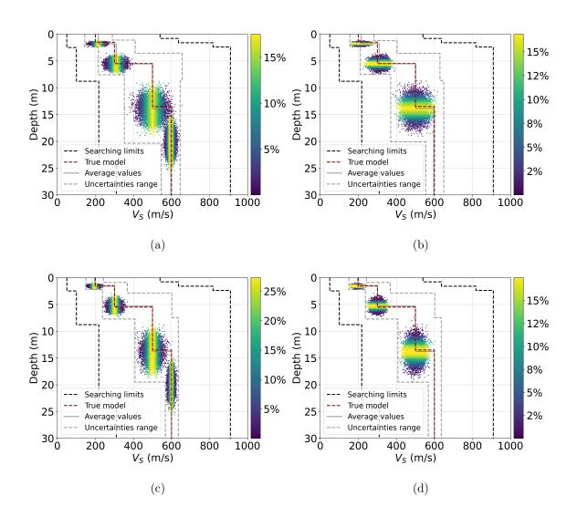
Figure 4: Results of uncertainty quantification for PGV-model: S-wave errors distributions (a) and thickness errors distributions (b) by uni-mode inversion and S-wave errors distributions (c) and thickness errors distributions (d) by multi-mode inversion. Color scaling means the percentage of hit rate in pixel.
