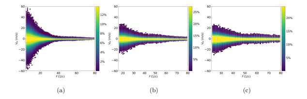
Figure 2: The noise data distributions for fundamental (a), first (b) and second (c) modes extracted from the phase velocity dispersion curves for PGV-model. Color scaling means the percentage of hit rate in pixel (the brighter it is, the more hits it has).
