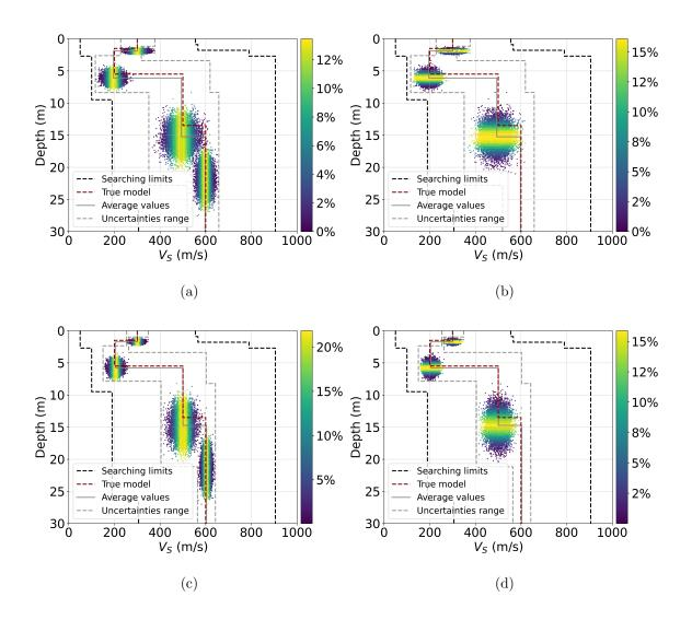
Figure 7: Results of uncertainty quantification for LVL-model: S-wave errors distributions (a) and thickness errors distributions (b) by uni-mode inversion and S-wave errors distributions (c) and thickness errors distributions (d) by multi-mode inversion. Color scaling means the percentage of hit rate in pixel.
