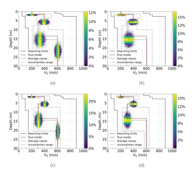
Figure 9: Results of uncertainty quantification for HVL-model: S-wave errors distributions (a) and thickness errors distributions (b) by uni-mode inversion and S-wave errors distributions (c) and thickness errors distributions (d) by multi-mode inversion. Color scaling means the percentage of hit rate in pixel.
