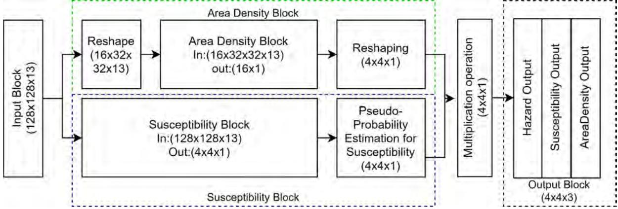
Figure 5: Designed landslide susceptibility and area density prediction model
