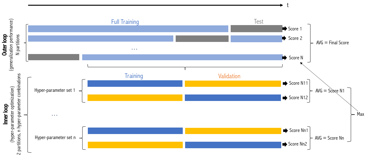
FIG. A1: Nested cross-validation scheme Figure adopted from Vabalas et al. (2019).
