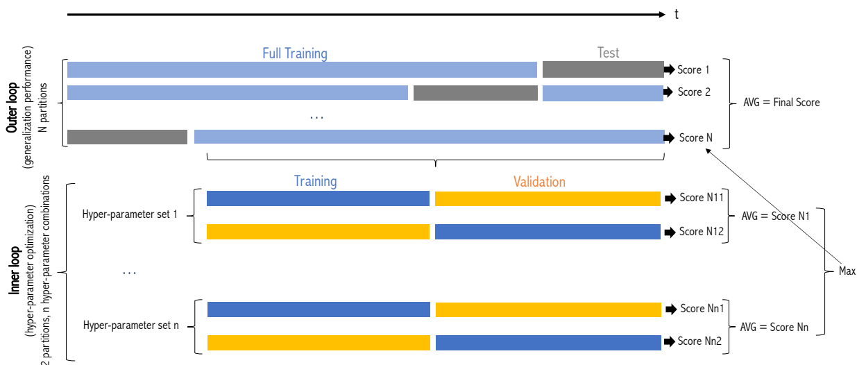
FIG. B1. Nested cross-validation scheme. N = 5 different test sets are predicted by the statistical models and the metrics with respect to the ground truth are calculated for each test set. The final metrics are obtained by averaging the metrics for the five test sets. The uncertainties of these metrics are estimated via the standard deviation of these 5-member ensembles. This figure is adopted from Vabalas et al. (2019).
