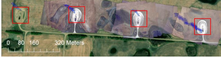
28 29 30 31 32 33 34 Figure S1: Four inactive, previously oil-producing, facilities used for high-flowrate controlled releases to study Bridger Photonics Inc.'s Gas-Mapping LiDAR technology. The four facilities were approximately 375 m apart in the west-east direction and less than 100 m in size in the north-south direction, permitting measurement of four controlled releases in rapid succession.
