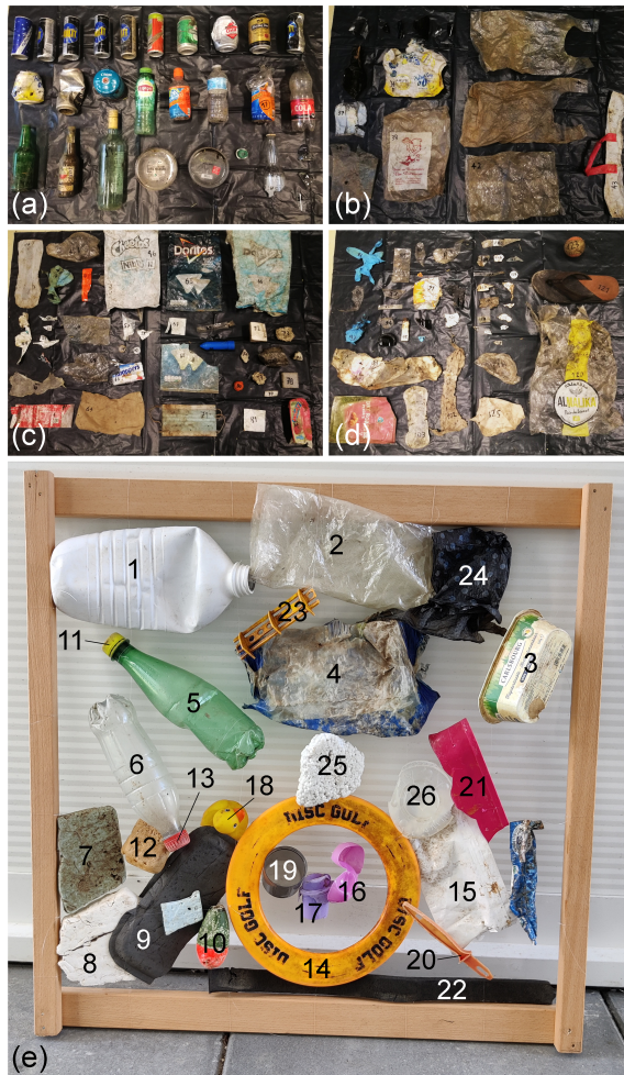
Figure 1: Riverbank-harvested items from Rhenen used for hyperspectral imaging in controlled environment (a-d); frame with riverbank-harvested items from Maastricht used for hyperspectral imaging in natural environment (e).
