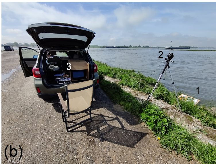
Figure 2: Hyperspectral imaging setup used by Tasseron et al. [5] (a); Hyperspectral imaging setup in the natural environment (b) with riverbank-harvested sample items (1), IMEC Snapscan SWIR hyperspectral camera (2), laptop with data capture software and power source (3).
