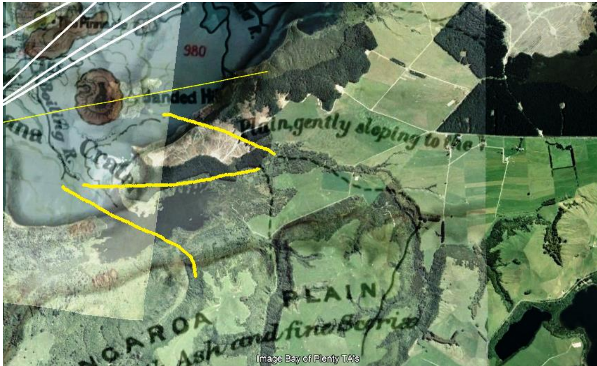
Fig. 9: Georeferencing showing Boiling River branches superimposed over Hangapoua Stream on Hochstetter's manuscript map. It connects with streams 1283784 and 1283810. The Waiahinekahu connects to the existing stream 1102186. Note the three eastern gullies, issuing these streams then and now.
