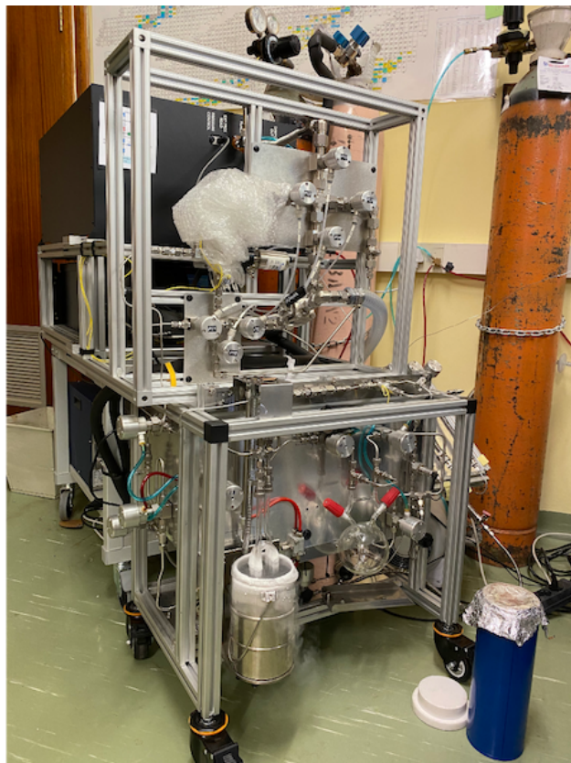
Figure 5: Photograph of the TILDAS instrument (lasers housed inside black box), with automated valve sampling system (top), and custom-built cart for automated CO 2 extraction and dilution (below).
