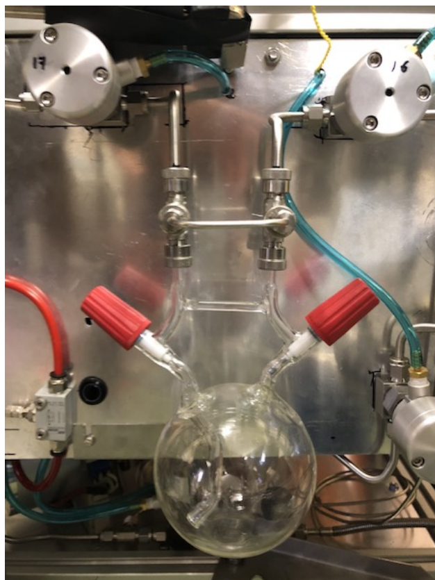
Figure 7: Photograph of MV1, the custom-built sampling flask (GlassChem cc, South Africa). Two teflon stopcocks (either Schott Produran or J. Young) seal off a \sim 586 mL round-bottomed borosilicate flask. A siphon ensures efficient flow through the volume. The flask can be disconnected from two Ultra-Torr quick connects (Swagelok). Valves 17 and 16 are shown to the left and right of the flask, respectively. A short tube of 1/8 " diameter acts as a bypass for the flask. All other tubes are 1/4 ". The piece of horizontal glass on the flask parallel to this bypass tube is solid, and is used to carry the flask when disconnected from the autocart. A design drawing for the flask can be obtained from the author upon request.
