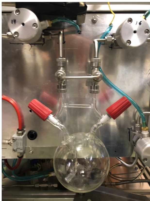
Figure S3: Photograph of MV1, the custom-built sampling flask (GlassChem cc, South Africa). Two teflon stopcocks (either Schott Produran or J. Young) seal off a \sim 586 mL round-bottomed borosilicate flask. A siphon ensures efficient flow through the volume. The flask can be disconnected from two Ultra-Torr quick connects (Swagelok). Valves 17 and 16 are shown to the left and right of the flask, respectively. A short tube of 1/8 " diameter acts as a bypass for the flask. All other tubes are 1/4 ". The piece of horizontal glass on the flask parallel to this bypass tube is solid, and is used to carry the flask when disconnected from the Autocart. A design drawing for the flask can be obtained from the author upon request.
