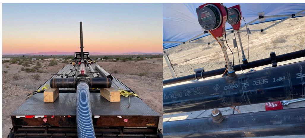
Figure 5. Metering and release trailer (left) has four pipes (0.5-inch, 2-inch, 4-inch, and 8-inch), each leading to a distinct metering location allowing a different dynamic range of release volumes. The three larger pipes used a QuadraTherm 640i insertion meter (right), with upstream 8.5 m straight run of pipe to ensure sufficient flow stabilization for all pipes. The 0.5-inch pipe was not used in this study.
