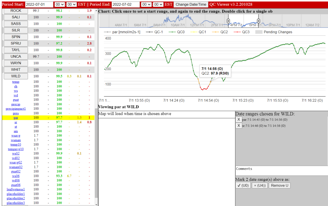
435 Fig. 4. ECONet Quality Control Data Viewer (QCDV) graphical user interface window 436 showing photosynthetic active radiation (PAR) observations at the Williamsdale Field Lab 437 ECONet station (WILD) in Wallace, North Carolina on July 1, 2022. Left panel shows results for 438 all stations and each individual sensor and the right top panel shows the time series plot for the 439 selected sensor measurement variable (e.g., PAR) with observations colored by quality control 440 score. Right bottom panel shows a map, any manual quality control notes, and user flag indicator 441 selection. User notes and user flags provide more context in manual quality control processing 442 (Section 5.2). Orange or red points in the time series indicate observations that have a quality 443 control (QC) score of two or three, respectively, and need further investigation.
