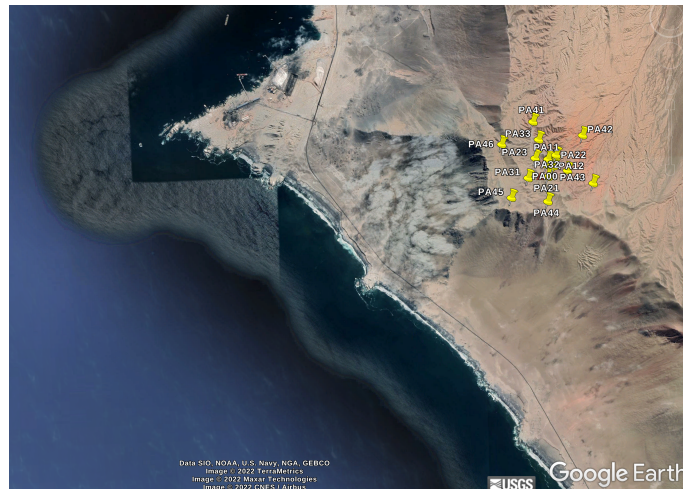
Figure 1. Screenshot of the array in Google Earth. The yellow pins stand for the PESCO stations. The picture highlights the cliff escarpment. The shoreline orientation is in agreement with the beamforming results in which the noise strikes the array from a south-west direction.
