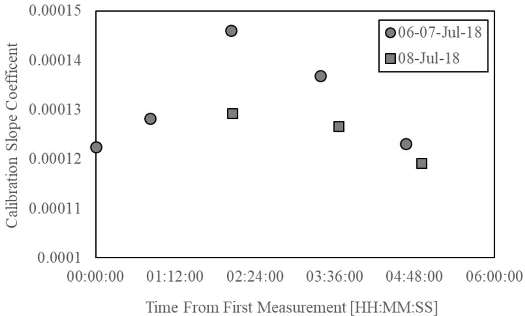
**Figure 4:** Example calibration slope coefficients from two days of data. Timings are from the time of the first calibration on each of these measurement days. Note that the data peaks towards solar noon.
