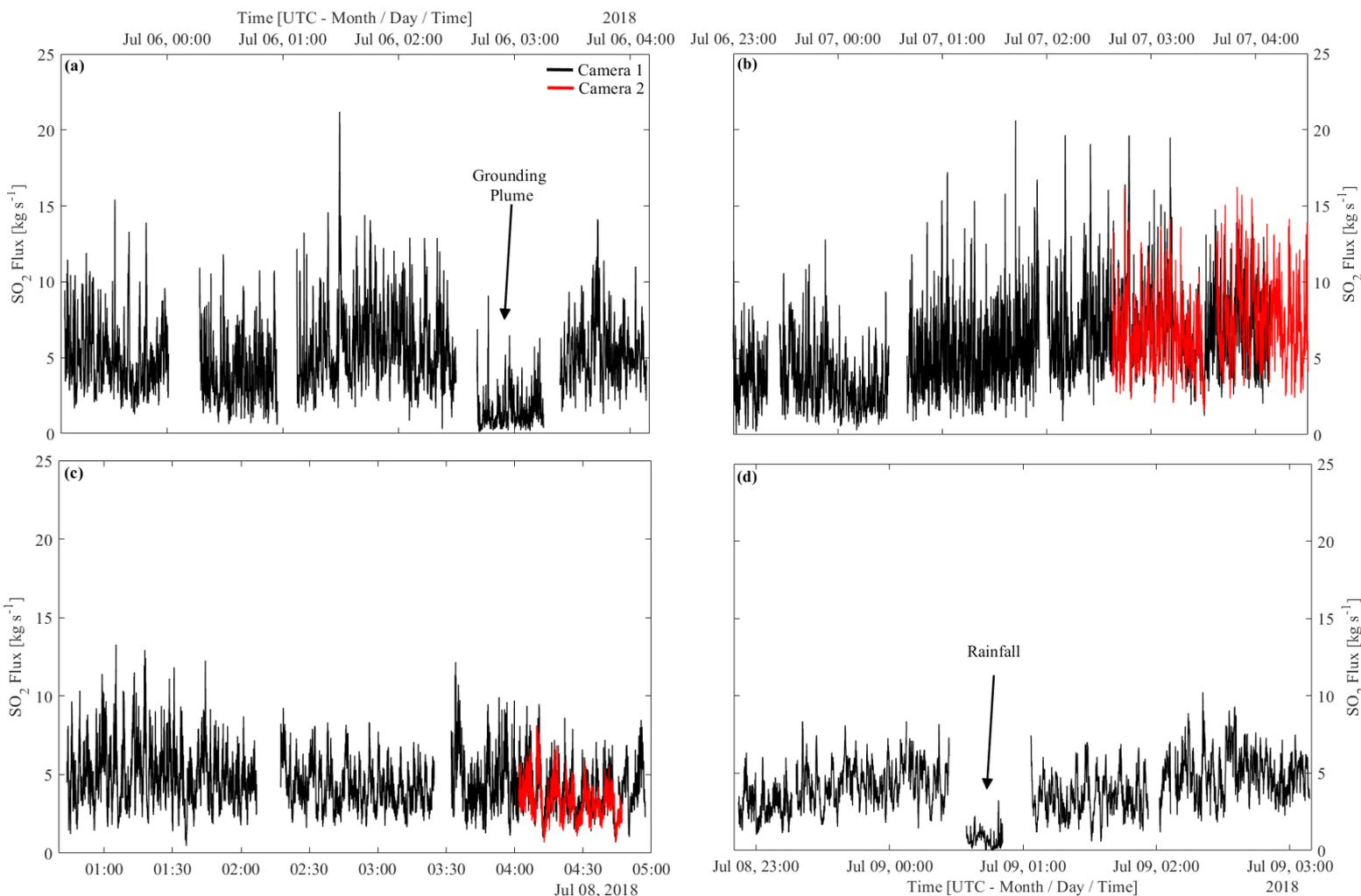
**Figure 6:** (a) through (d) show retrieved gas fluxes for all the image data captured during the observation period; also highlighted are periods where the plume was grounded in (a) and heavy rainfall was encountered in (d).
