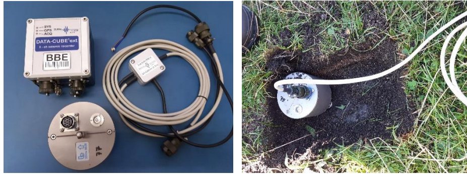
Figure 2. Seismic instruments used throughout the fieldwork. (a) Three-component (3C) Lennartz short-period 1Hz seismometer, data-cube digitizer and breakout-box to connect the seismometer to the data-logger, (b) deployment of a seismometer in a 30cm deep pit to alleviate the effect of cultural, wind and rain noise.
