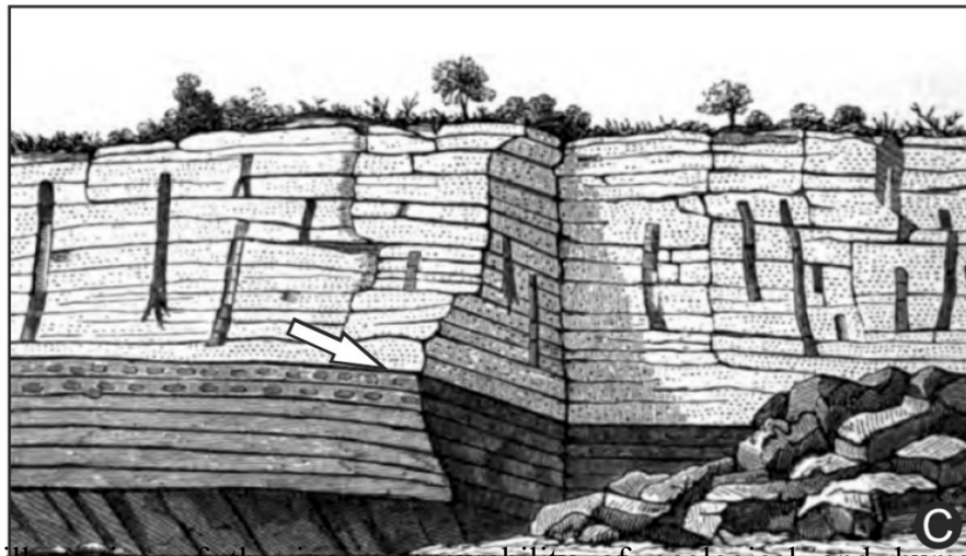
Figure 2. An illustration of the incommensurability of geological and human time scales: Pennsylvanian trees buried in position of growth. These “polystrate” fossils document rapid sediment accumulation at the scale of days to years that cannot be maintained through any geologically significant length of time, and thus must be compensated by long periods of non deposition concealed in a series of subtle discontinuities such as those indicated by arrows. A) Nant Lech, Swansea Valley, South Wales (fig.4.5 in Ager 1993 ); B) Joggins, Nova Scotia (fig.35 in Dawson, 1868 ); C) St. Étienne, France (fig.310 in Credner, 1906 ).
