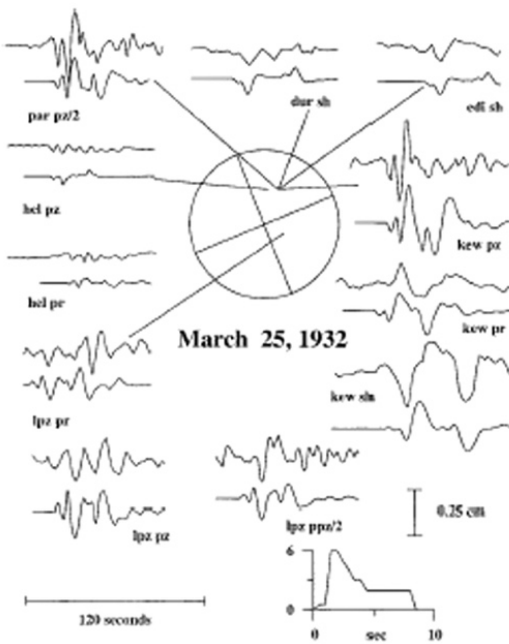
Figure 1. Analysis of the MW 6.8 Prince William Sound earthquake of March 25, 1932 by Doser and Brown (2001). Observed seismograms (top) and synthetic seismograms (bottom). Labels shown below seismograms refer to station code and waveform type (pz, vertical P; pr, radial P; sh, transverse S; pp, PP phase). Vertical scales show seismogram amplitudes in cm. Inset source time function plots have amplitudes of 10^{18} N m/sec. First motion data that were used to help constrain the inversion process are shown.
