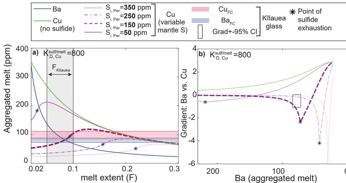
Figure A11: Models for  $S_i=350, 250, 150$  and  $50$  ppm. Although the  $S_i=150$  ppm model scenario recreates observed Cu concentrations, if sulfides are exhausted, it doesn't mass through observed gradients or Ba concentrations.
