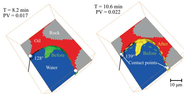
**Figure 4.** Visualisation of a detail of the pore space where we can observe the pinning of the oil-brine interface. During water injection, while the three-phase contact points (white dots) did not move, the interface changed its shape (from green to yellow), with a consequent increase in contact angle. Pore volumes (PV) were computed considering the total macro pores of the whole sample.
