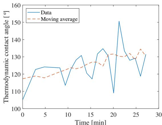
**Figure 9.** Thermodynamic contact angle, computed using Eq. (3.1) between two subsequent time steps. The 3-points moving average (dashed line) shows the increasing trend as the displacement proceeds.
