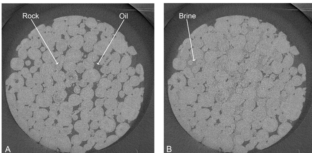
**Figure 1.** 2D slices of the 3D tomograms as they appear after reconstruction. Panel A shows a slice of the image before water injection, while the image in panel B was taken at the end of water injection.
