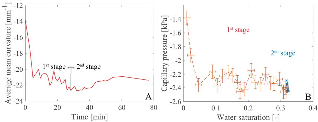
**Figure 7.** (A) Average mean curvature of the oil-water interface, (B) capillary pressure, before (dashed red line) and after (blue crosses) breakthrough.
