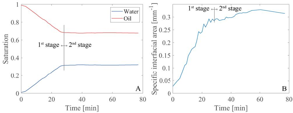
**Figure 6.** (A) Change in time of water and oil saturation, (B) specific interfacial area between oil and water.
