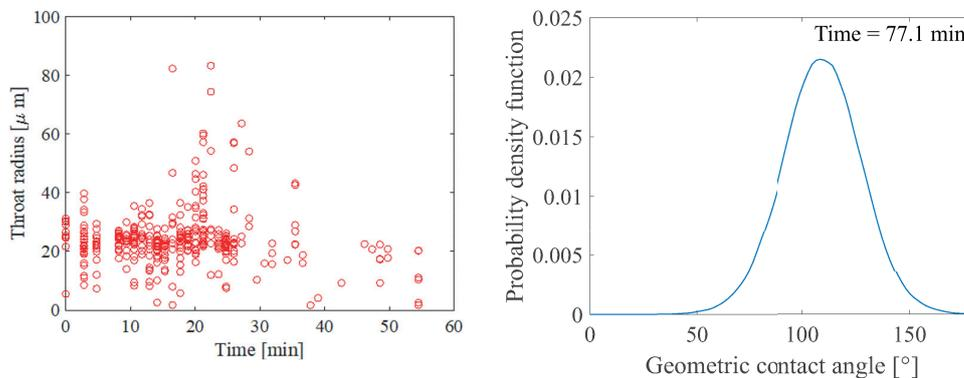
**Figure 5.** (A) Scatterplot where the radius of invaded throats is the dependent variable and the time at which they were filled is the independent variable. (B) Geometric contact angle between water and oil at the end of waterflooding.
