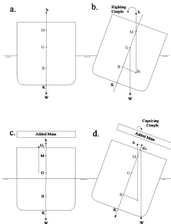
When a vessel is built, the position of her initial metacentre is determined by an inclining experiment and the height of the metacentre above the keel (KM) is tabulated for different draughts. To ensure all vessels are stable enough to meet all expected
