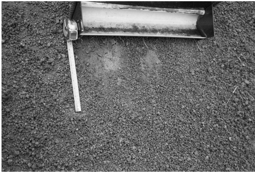
Fig. 5. Particles and soil surface are washed out around the splashboard.
