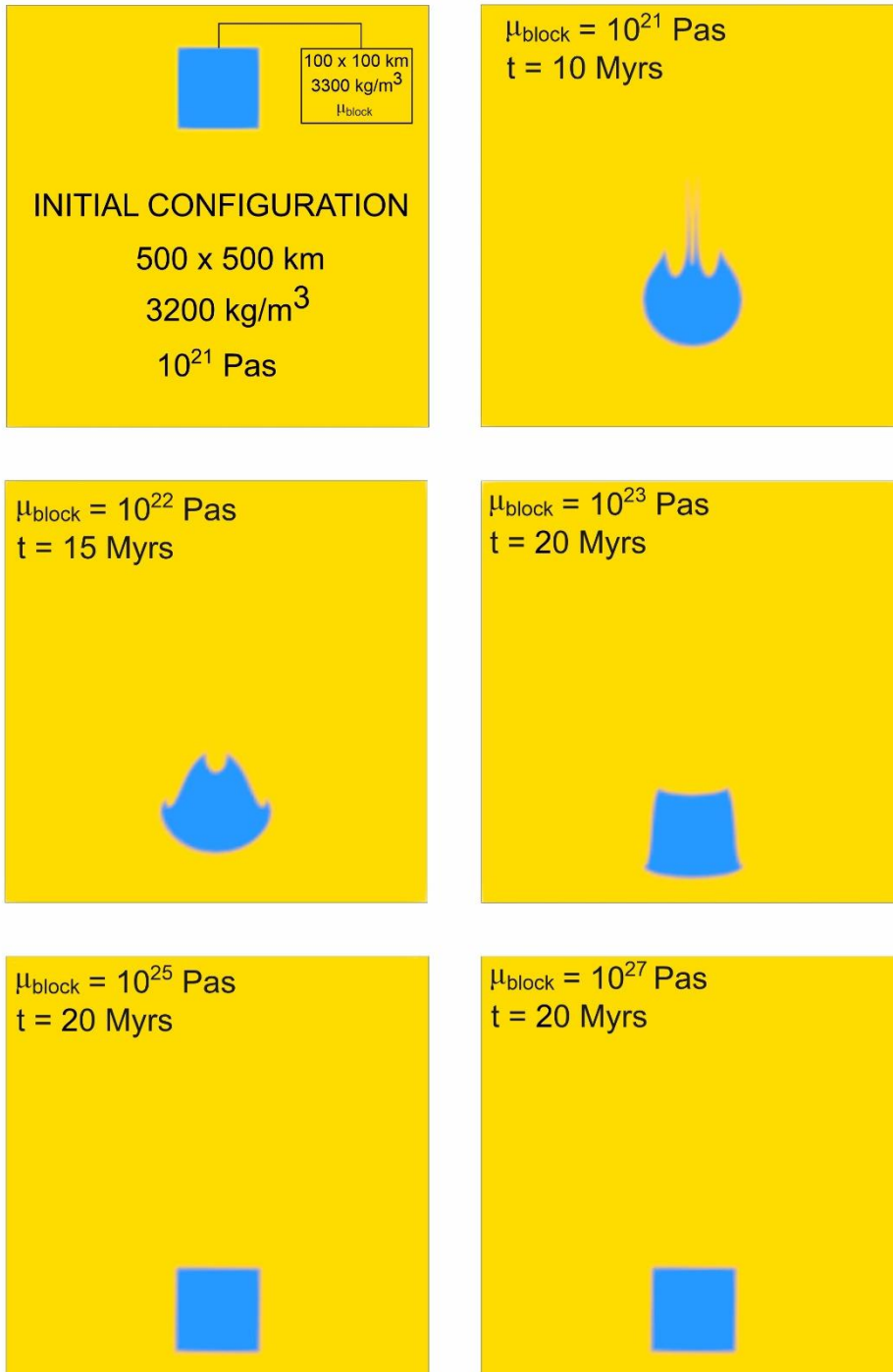
Figure A1: Falling-block benchmark experiments for \Delta\rho = 100 \text{ kg/m}^3 . Initial model conditions are shown in the top left panel. Note that the degree of block deformation decreases with increasing block viscosity (indicated top left corner of each panel, which match well with the previous simulation results (Gerya, 2010; Thieulot, 2011))
