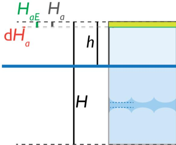
**Figure 8.** Cartoon graphic showing relevant quantities for a column of ice floating in seawater. The ice below sea level is discontinuous to exaggerate the vertical scale. Quantities represent observed or accepted values as in Fig. 2, with added  $H_{aE}$ , which is the firm air column thickness necessary to bring the observed ice column into hydrostatic equilibrium, and  $dH_a$ , which is the difference between  $H_{aE}$  and the modeled firm air column thickness  $H_a$ .
