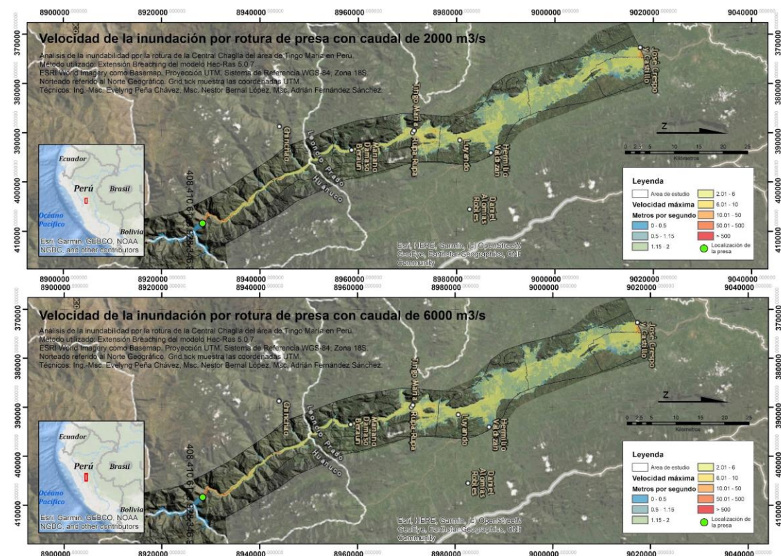
Figure 6. Simulated maximum velocities for flooding due to breaching of the Chaglla dam.
