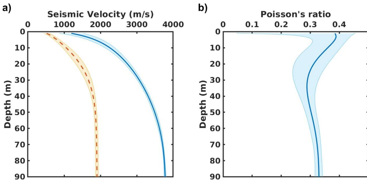
**Fig. 5.** a) Results from Wiechert-Herglotz inversion, showing the depth-dependence of seismic P-wave (blue solid line) and S-wave (red dashed line) velocity. b) Poisson's ratio as a function of depth in the firn column. Shaded areas indicate uncertainties.
