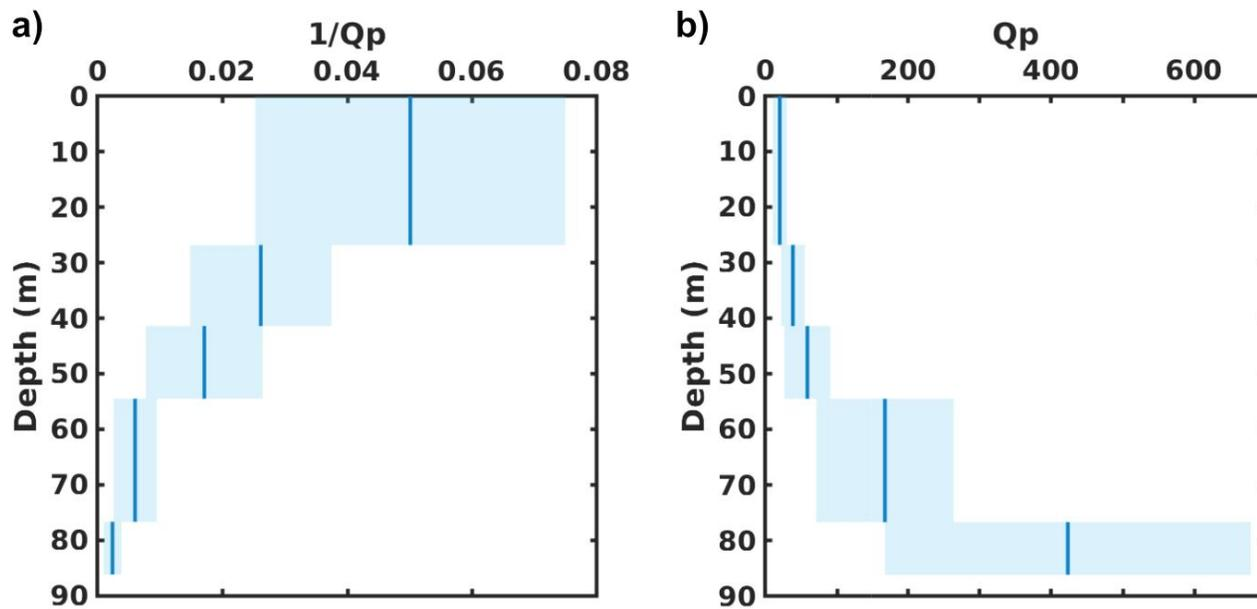
**Fig. 6.** a) Mean of  $1/Q_p$  versus depth for a five-layer model. Shaded area represents the standard deviation of sampled models. b)  $Q_p$  model resulting from statistical analysis of  $1/Q_p$  data.
