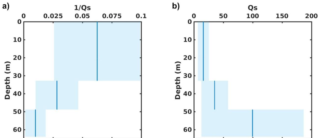
**Fig. 7.**  $Q_s$  results. a) Mean  $1/Q_s$  for each layer with standard deviation shaded. b)  $Q_s$  model resulting from  $1/Q_s$  calculations.
