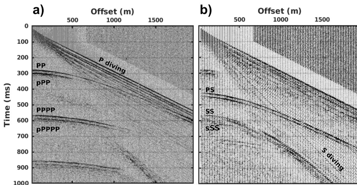
**Fig. 2.** Aggregated shot gathers in the a) vertical and b) radial directions, with automatic gain control applied for inspection only. Primary reflections (PP, SS) and their surface ghost reflections (pPP, sSS) are clearly visible, as well as multiples and their ghosts (PPPP, pPPPP), a converted wave reflection (PS), and the P and S diving waves.
