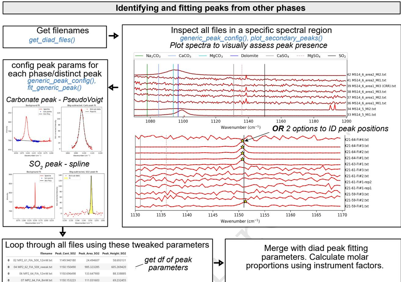
Figure 4: Schematic of workflow used to fit secondary peaks (e.g., carbonate, SO<sub>2</sub>). Secondary peak fitting results are then merged with diad parameters (allowing calculation of molar proportions of gas species).
