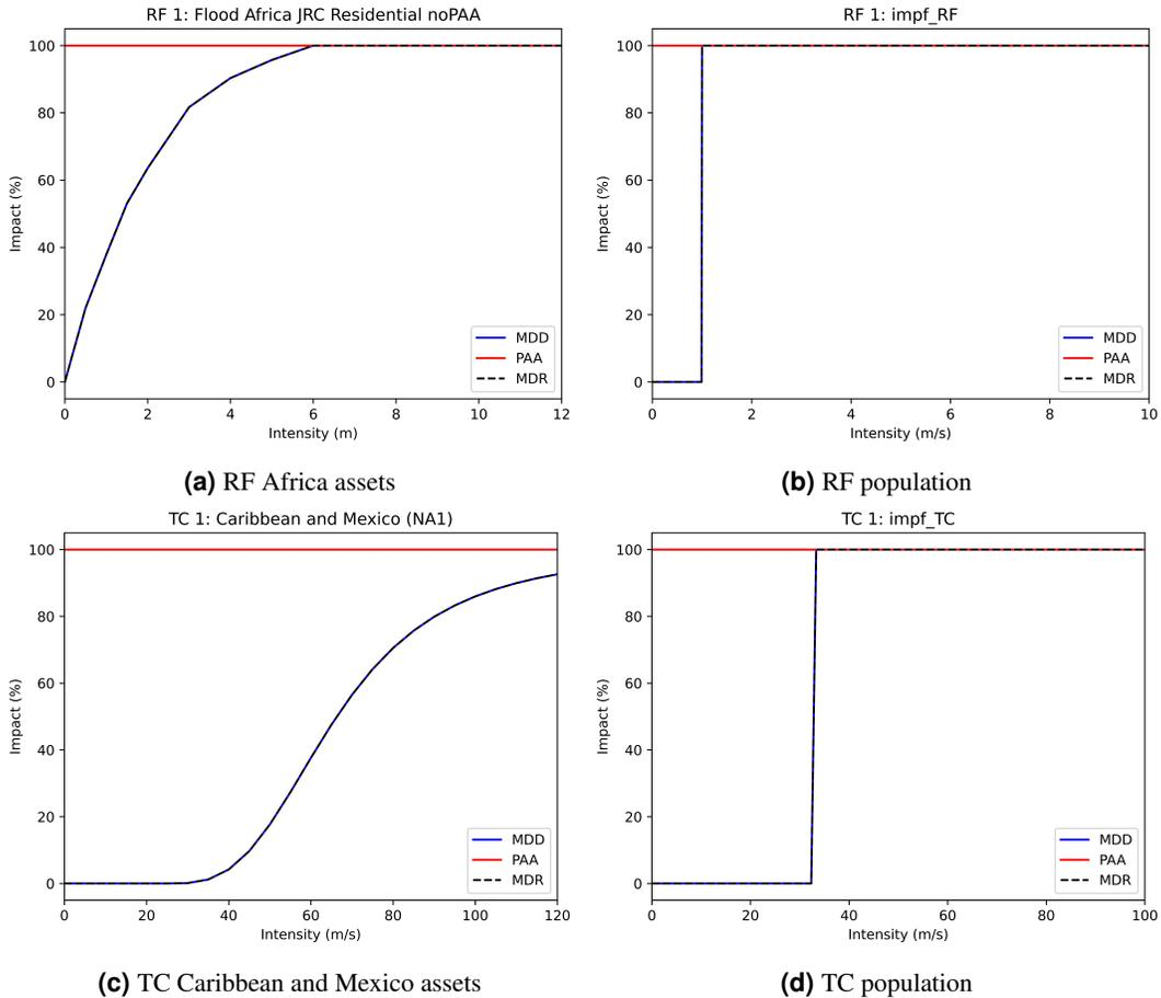
**Supplementary Figure 5.** Example of impact functions used in the impact calculation. In the case of assets, vulnerabilities are separated in 10 regions, while for RF there are a total of 6 regions. In the case of population, one function is used per hazard with a threshold.
