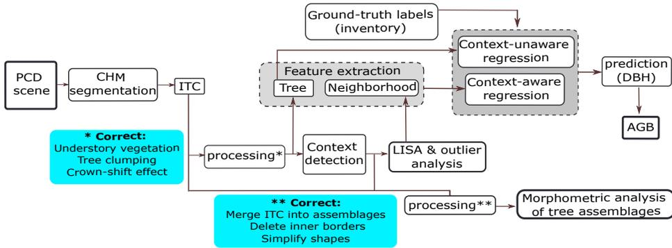
**FIGURE 3** Workflow followed in this study. PCD: point cloud data, CHM: canopy height model, ITC: individual tree crown, LISA: local indicators of spatial association, DBH: diameter at breast-height, AGB: aboveground biomass. The two colored boxes describe the subtasks constituting each of the processing steps, marked \* and \*\* in the diagram.
