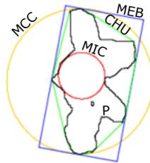
**FIGURE 10** Calculation of elementary geometries fitted to an exemplary tree assemblage. P: polygon of tree assemblage (black line). MCC: minimum circumscribed circle (in green). MIC: maximum inscribed circle (in red). CHU: convex hull (in yellow). MEB: minimum enclosing box containing P (in blue).
