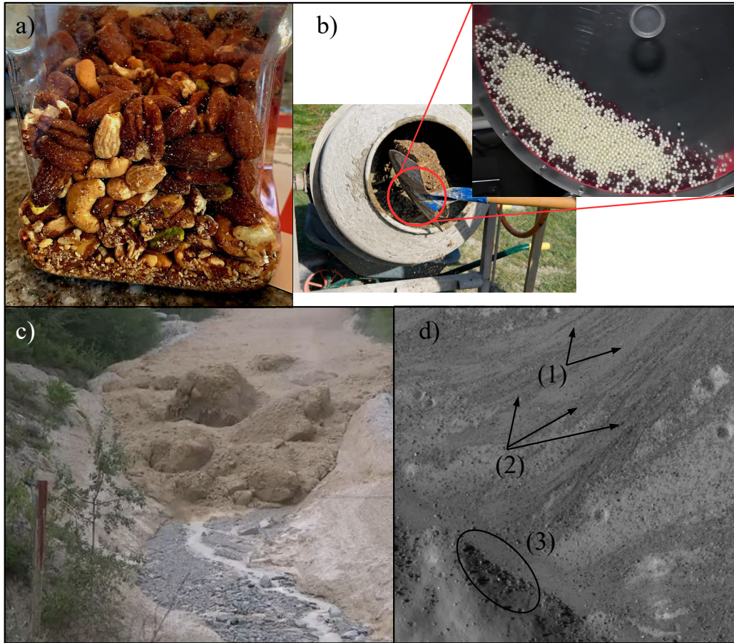
Fig. 1. Processes of granular segregation. (a) Brazil nut effect in a jar of nuts. (b) Process of mixing cement. Inset: Granular mixture in a rotary drum composed by marbles with diameters of d_s = 4 and d_b = 8 mm. (c) Granular segregation in the front of the Illgraben debris flow. Photo by Pierre Zufferey. Image credit: American Geophysical Union. (d) Debris flow deposit-terminations in Kepler moon crater (latitude 8.32^\circ\text{N} , longitude 37.69^\circ\text{W} )(20). (1) Finer-grained fractions (fines), (2) coarse dark levees, and (3) terminal deposits.
