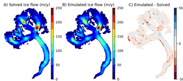
**Fig. 15.** Surface ice flow field of Aletsch Glacier with the parameters found after performing the simultaneous inversion and emulator training: A) using the solver B) using the retrained emulator. Panel C) shows the spatial difference between the two.
