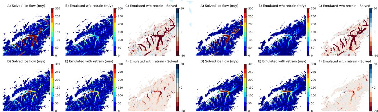
**Fig. 12.** Results of the ELA-varying (left panels) and A/c-varying (right panels) transient modelling experiments for Valais Glacier. Similar to the caption of Figure 10.
