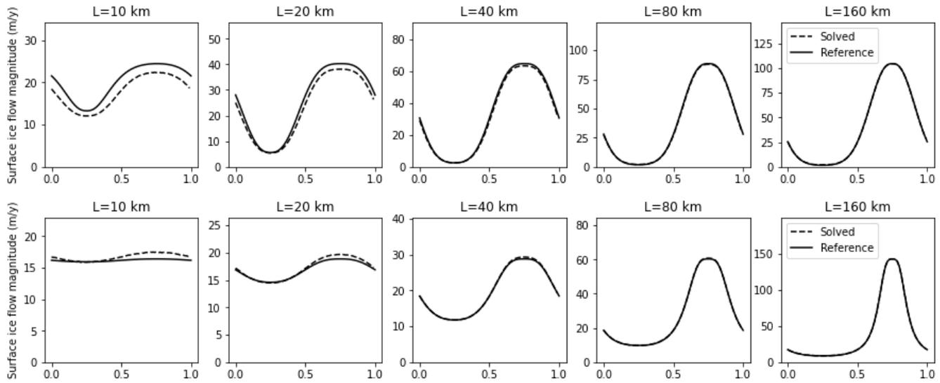
**Fig. 5.** Surface ice flow magnitude along the  $y = L/4$  horizontal line for different length scales  $L = 10, 20, 40, 80,$  and  $160$  km in the ISMIP-HOM experiments A and C: comparison between “solved” with reference solution ‘ogal’ obtained from Pattyn and others [2008]. For simplicity, the x-axis was scaled with  $L$ .
