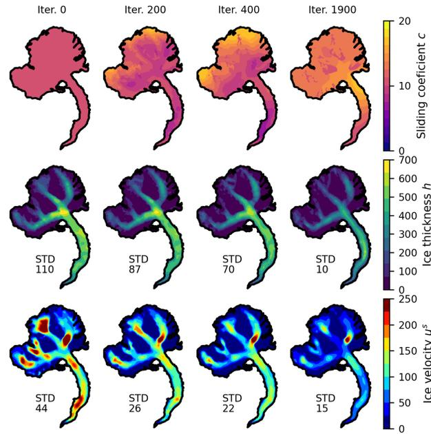
**Fig. 14.** Evolution of the sliding distribution  $c$  (unit:  $\text{km MPa}^{-3} \text{a}^{-1}$ ), the ice thickness distribution  $h$  (unit: m), as well as resulting surface ice flow velocity field  $\mathbf{u}^s$  (unit:  $\text{m y}^{-1}$ ) through the iterations of the optimisation problem for Aletsch glacier. The STandard Deviation (STD) between the modeled and observed fields is reported at each step.
