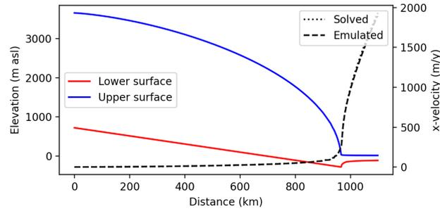
**Fig. 16.** MISMIP-inspired ice geometry of the ice shelf experiment along the  $x$ -axis, and resulting ice flow velocities modelled from the solver and the emulator with custom training on the specific geometry.
