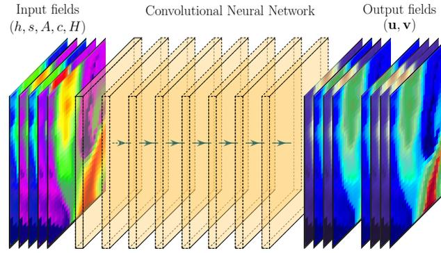
**Fig. 3.** Our emulator consists of a CNN that maps geometrical (thickness and surface topography), ice flow parameters (shearing and basal sliding), and spatial resolution inputs to 3D ice flow fields.
