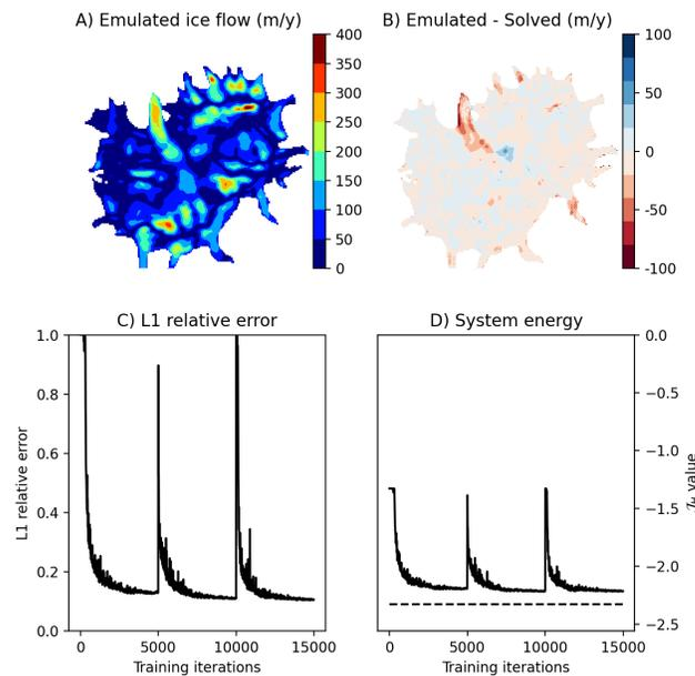
**Fig. 7.** Results of the emulator on the “test” glacier: A) “Emulated” surface ice flow at the surface of the test glacier (Fig. 6) at convergence of the offline training over the catalogue, B) difference between the “emulated” and “solved” solutions C) evolution of the L1 relative error between the two solutions and D) of the system energy through the training epochs.
