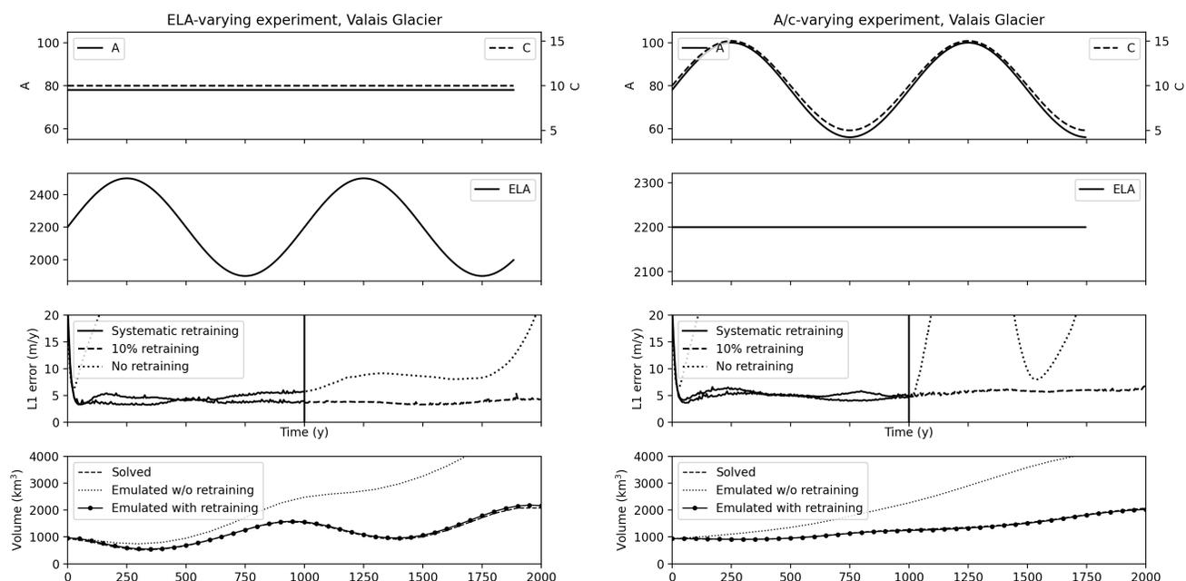
**Fig. 11.** Transient results of the ELA-varying (left panels) and A/c-varying (right panels) transient modelling experiments for Valais Glacier. This is similar to the caption of Figure 9.
