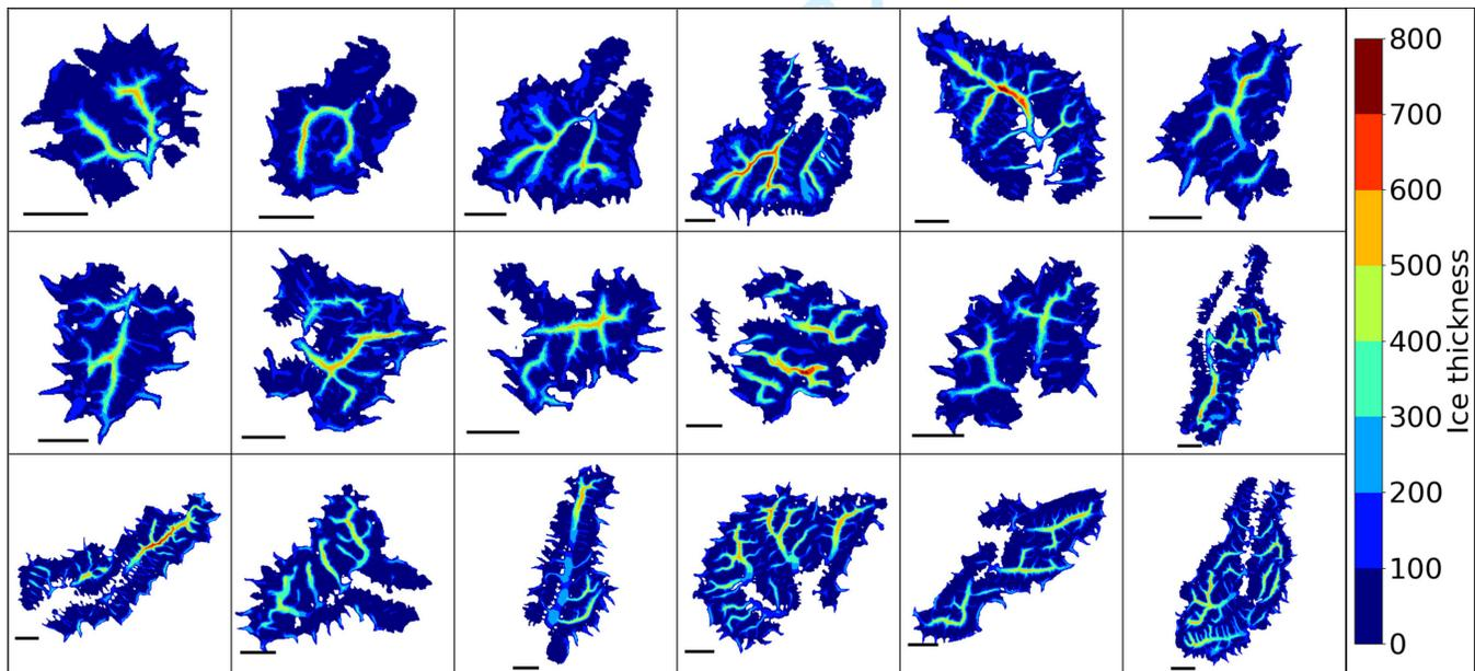
**Fig. 17.** Ice thickness at their maximum extent of half of the glacier catalogue (18 of the 36). Each glacier shape is a snapshot of a simulation initialised with ice-free conditions, and forced with a surface mass balance that permits building and retreat successive phases over a total of 200 years. The horizontal bar represents 5 km to give the scale of each glacier.
