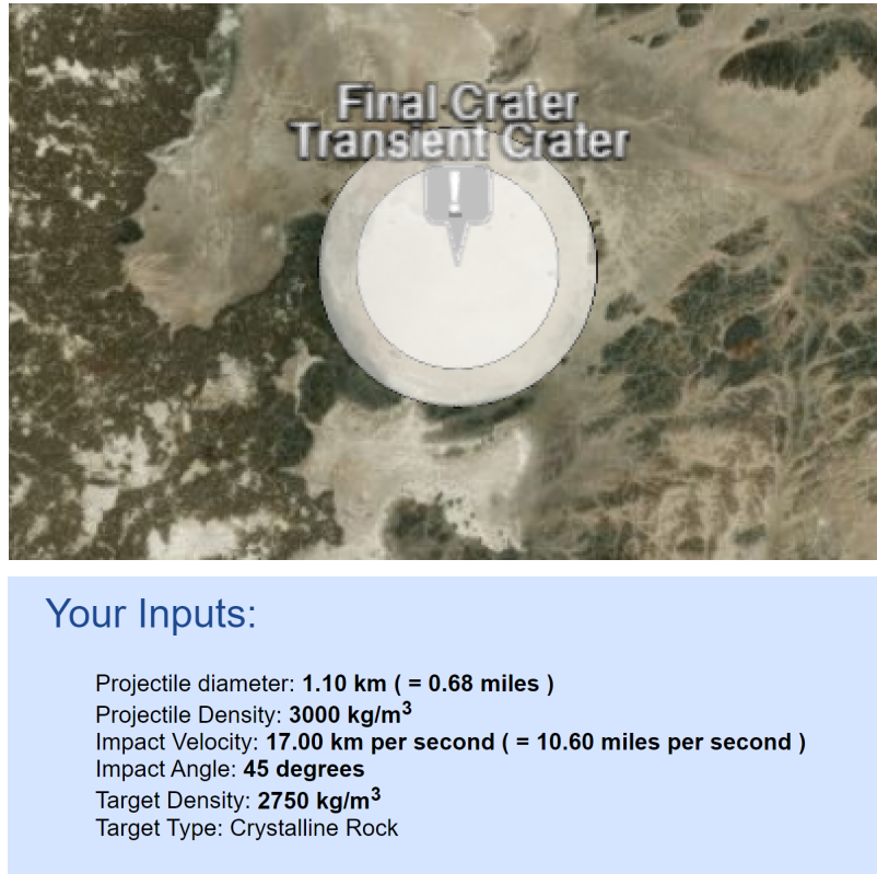
Figure 6: Figure 6 is a simulation conducted using the Impact Crater Map (Imperial College London) made by Gareth Collins, Robert Marcus, H.J Melosh.
