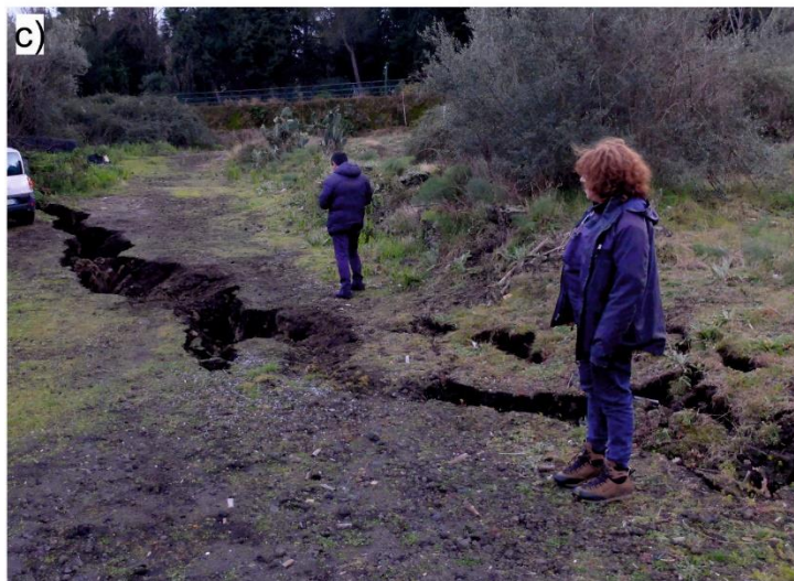
242 FIGURE 3: FIELD PHOTOS OF GROUND CRACKS IN ASPHALT AND PAVED ROADS (A, B) AND SOILS (C, D). LOCATION IS SHOWN IN 243 FIGURE 2.
