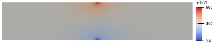
Figure 4: Distribution of the electrical field in the sample between the electrodes placed in the center at the top and bottom of the sample. The time step shown is 2 \mu s following the electrical discharge.
