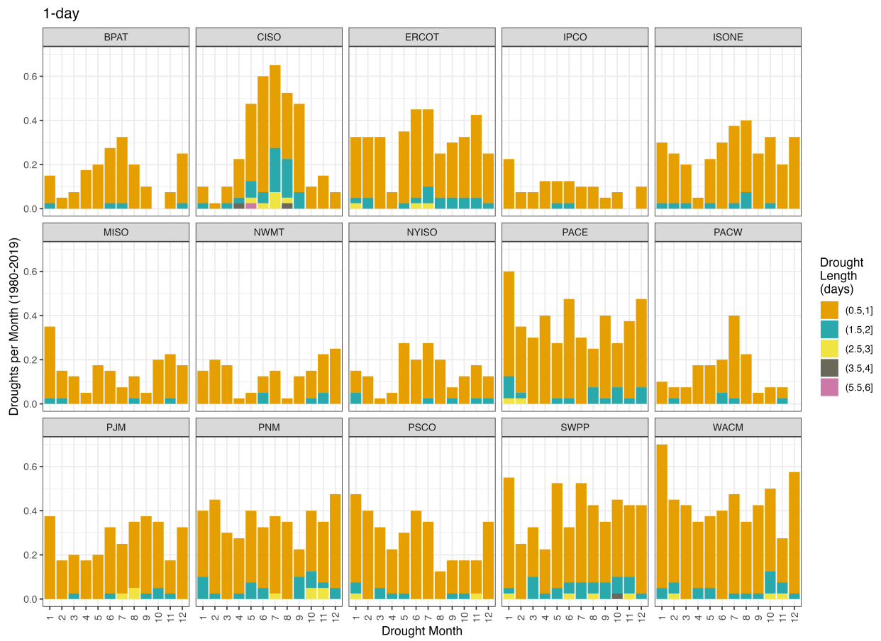
Figure 5: Seasonal distributions of energy droughts. The bar heights indicate the frequency of droughts in a particular month (average number of droughts per year). The color indicates the drought duration.
