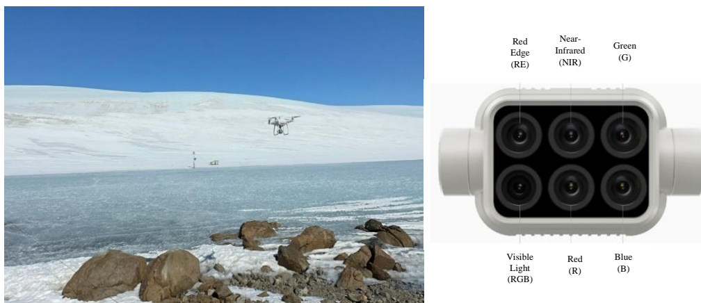
1036 Fig. 26. The UAV survey over the glacial lake with P4 multispectral sensor
