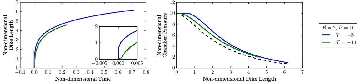
**Figure S5.** Dike length versus time and chamber pressure versus dike length with  $\mathcal{K} = 3$ ,  $\mathcal{B} = 2$ ,  $\mathcal{P} = 10$ , for  $\mathcal{T} = -5$  and  $\mathcal{T} = -10$ . In contrast to that with  $\mathcal{T} = -10$ , the case with  $\mathcal{T} = -5$  initially experienced unstable crack growth, growing to approximately 0.64 times the chamber radius.
