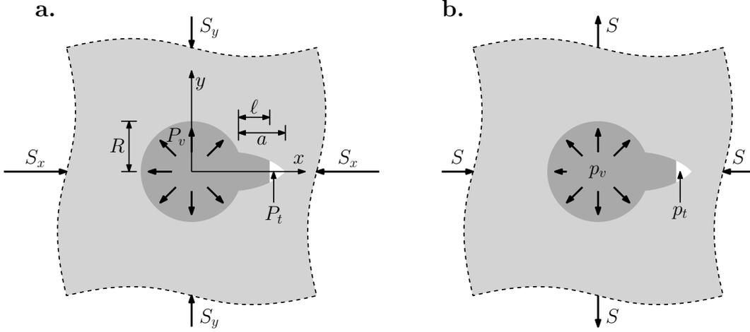
**Figure 1.** (a) Schematic of the radial dike problem. (b) Problem with mean stress subtracted. In both figures, the dike is depicted in the deformed configuration, exaggerating the opening of the dike.
