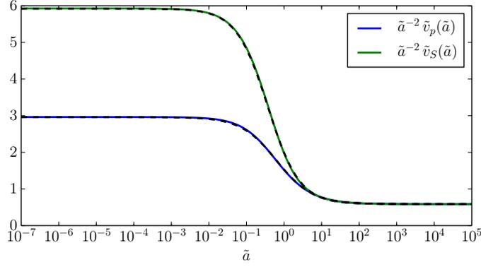
**Figure 4.** Non-dimensional crack volume functions for a circular hole with a straight edge crack subjected to unit far-field hydrostatic tension (blue curve) and deviatoric stress (green curve), computed using the elasticity solution of Tweed and Rooke (1973). Black dashed lines correspond to the approximations (6). For  $\tilde{a} < 10^{-2}$  and  $\tilde{a} > 10^1$ , the elasticity behavior is well approximated by an edge crack and an internal crack with no magma chamber, respectively.
