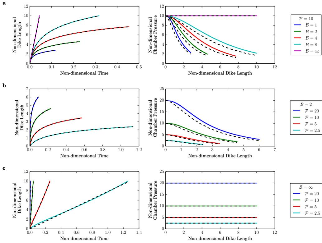
**Figure 2.** Dike length versus time and chamber pressure versus dike length for (a)  $\mathcal{P} = 10$  and varying  $\mathcal{B}$ , (b)  $\mathcal{B} = 2$  and varying  $\mathcal{P}$ , and (c)  $\mathcal{B} = \infty$  and varying  $\mathcal{P}$ . The fitted model for dike length versus time equation (3) and the simplified pressure versus dike length model equation (5) are shown with black dashed lines.
