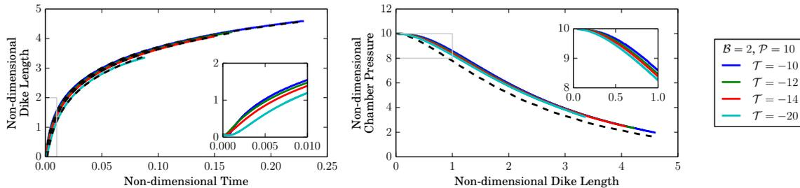
**Figure S4.** Dike length versus time and chamber pressure versus dike length for  $\mathcal{K} = 3$ ,  $\mathcal{B} = 2$ ,  $\mathcal{P} = 10$ , and varying  $\mathcal{T} \in \{-10, -12, -14, -20\}$ . Dashed lines indicate the log model (4) and depressurization model (6), which show good agreement with the data. (Left inset) Zoom of early-time behavior, showing initially slow growth for dikes with decreasing tip pressure. (Right inset) Closeup of the chamber pressure versus dike length.
