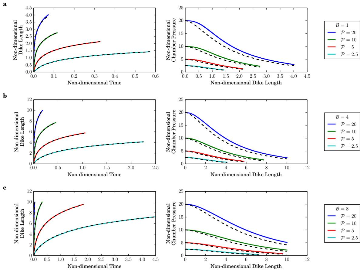
**Figure S2.** Dike length versus time and chamber pressure versus dike length for (a)  $\mathcal{B} = 1$ , (b)  $\mathcal{B} = 4$ , and (c)  $\mathcal{B} = 8$ , varying  $\mathcal{P} \in \{2.5, 5, 10, 20\}$ . The fitted logarithm model for dike length versus time and the simplified pressure versus dike length model are shown with black dashed lines.
