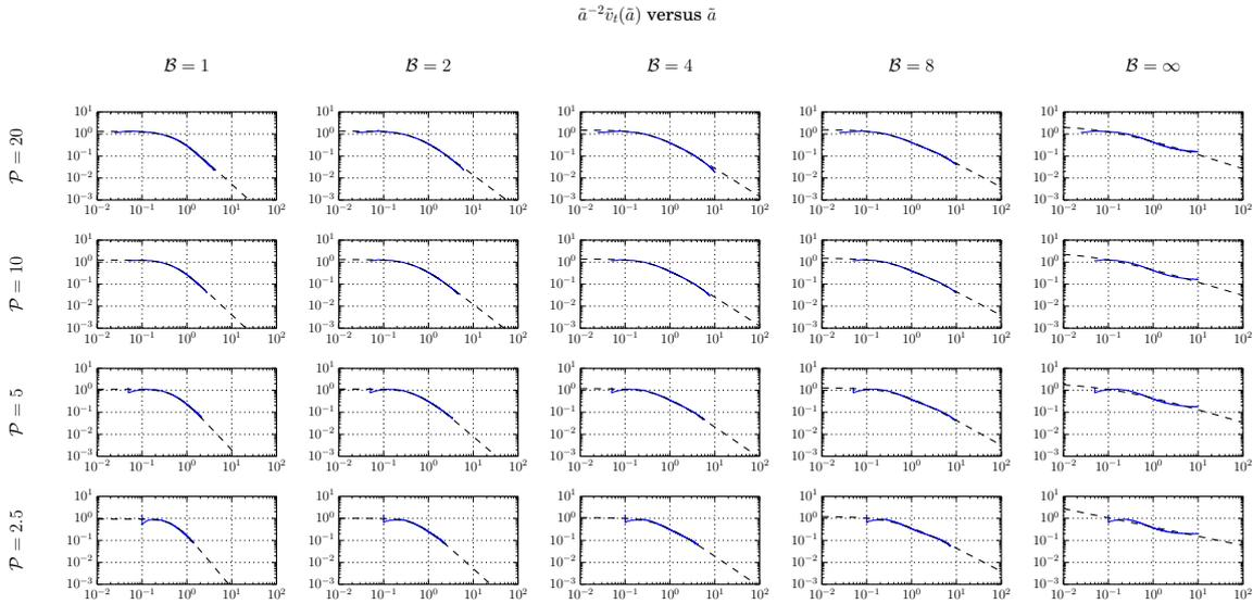
**Figure S6.** Tip cavity volume plotted against dike length over the explored parameter space. The numerical results are shown with blue lines, while the best fit of the functional form (8) is shown with dashed black lines. The model does not approximate well the cases with  $\mathcal{B} = \infty$ , which appear to have a limiting behavior  $\tilde{v}_t(\tilde{a}) \sim \tilde{a}^2$  for  $\tilde{a}/A^* \gg 1$ .
