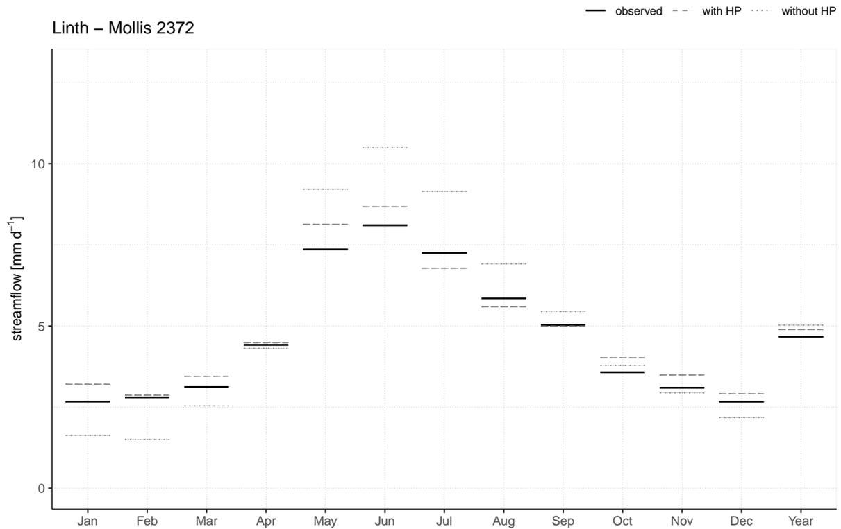
SI Figure 1: Hydropower impact in catchment I (Linth - Mollis 2372). The comparison of observed and simulated monthly mean streamflow. The black line represents the observed monthly mean streamflow, the dashed lines the simulated monthly means with and without consideration of hydropower, simulated with the hydrologic model PREVAH (section 3.2).
