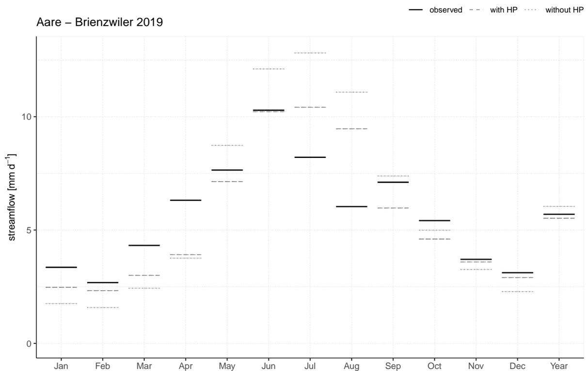
SI Figure 2: As Figure 1 but for hydropower impact in catchment II (Aare - Brienzwiler 2019).
