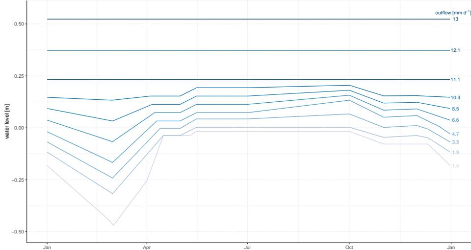
Figure 1: Example of a line diagram that defines a target outflow (blue lines) for each calendar day (x-axis) and for given lake water levels (y-axis).
