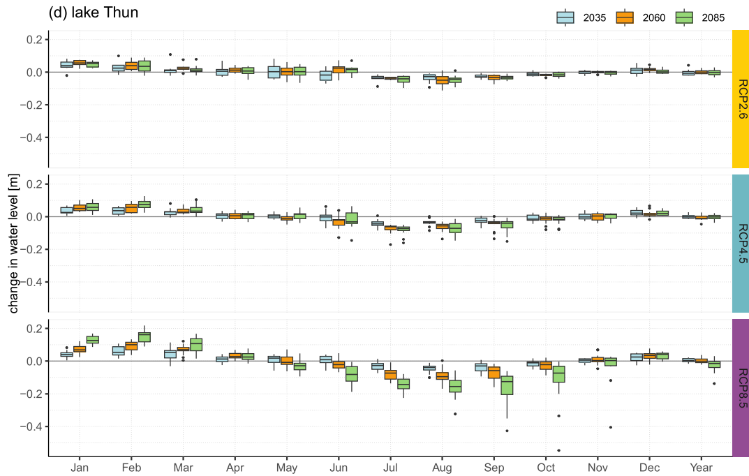
Figure SI 24: Simulated changes in monthly and annual mean lake levels of lake Thun, divided into the three future scenarios (2035, 2060, 2085) and three emission scenarios (RCP2.6, RCP4.5, RCP8.5).
