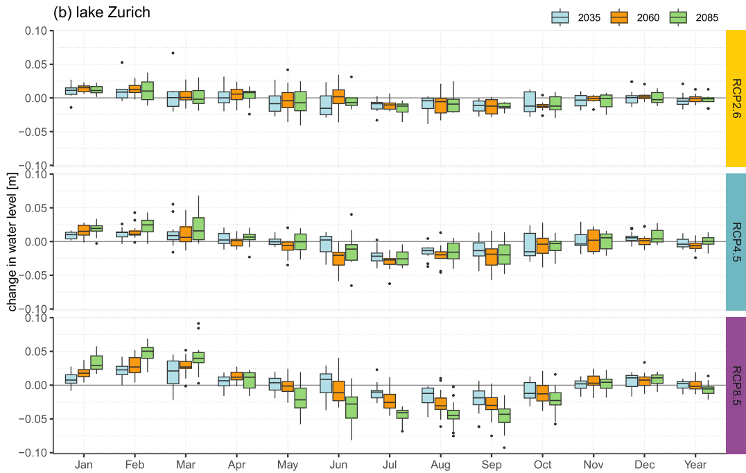
Figure SI 12: Simulated changes in monthly and annual mean lake levels of lake Zurich, divided into the three future scenarios (2035, 2060, 2085) and three emission scenarios (RCP2.6, RCP4.5, RCP8.5).
