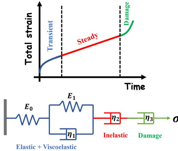
Figure 6: A simplistic general description of rock deformation mechanisms under a constant imposed stress  $\sigma$ . The parameters  $E_0, E_1$  are Young's modulus of elastic and viscoelastic elements and  $\eta_1, \eta_2, \eta_3$  are the viscosity of the elements.
