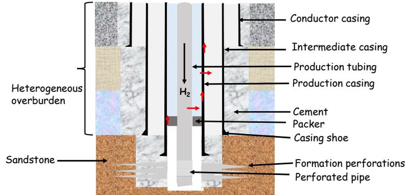
Figure 12: Simplistic illustration of a typical well indicating the possible  $H_2$  leakage pathways (red arrows) through the tubing, through inside and outside of the casing, and around the packer. Modified after [30, 48, 344, 345]. Additional pathways in the sheared well-bore and cement plug-in in the case of an abandoned well are not shown here.
