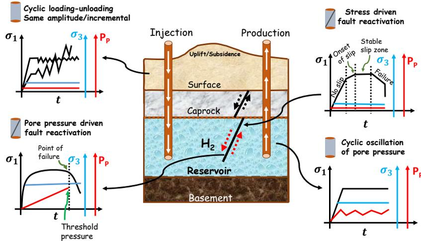
Figure 4: Illustration of the type of experiments being conducted in the laboratory scale relevant to UHS for the variation of different stresses ( $\sigma_1, \sigma_3$ ) and pore pressure ( $P_p$ ) with time ( $t$ ).
