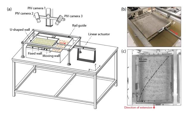
**Figure 2** (a) Experimental setup. (b) Oblique view photograph of the model (44 cm long and 40 cm wide) at the start of the experiment. (c) Top view photograph of the model surface (Exp LE-05) at the end of the experiment. The dashed line indicates the final geometry of the strong-normal basement boundary (see Fig. 3 for illustration of basement geometries). In all figures, the red arrow indicates the direction of extension.
