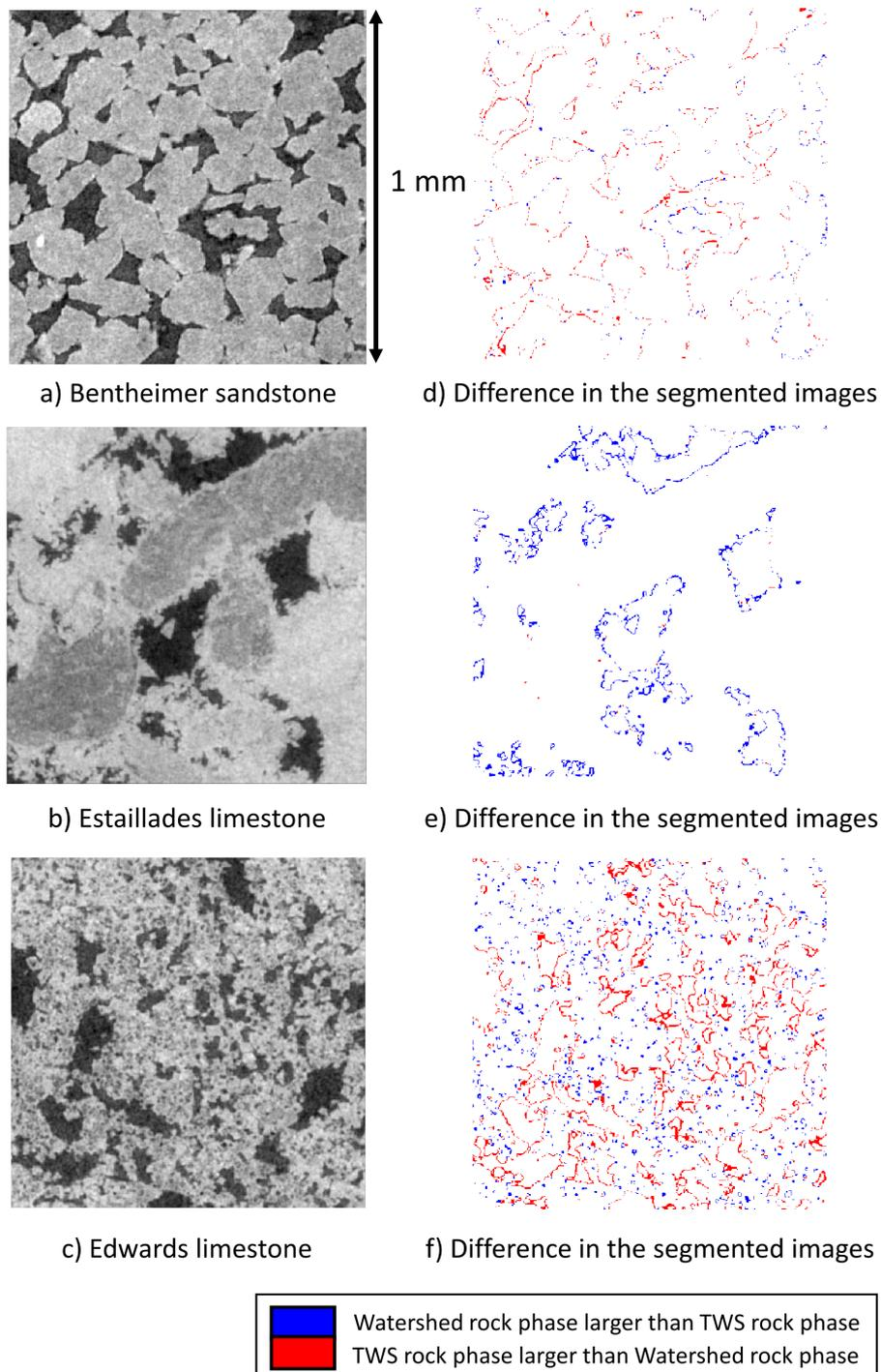
**Fig. 1** Cross sections of three of the five samples considered for the analysis of pore space properties sensitivity to image processing. The voxel size is  $2.5 \mu\text{m}$ . The rocks are, respectively: a) Bentheimer sandstone; b) Estailades limestone; c) Edwards limestone and the differential images obtained by subtracting the respective segmented images with the two processing pipelines considered.
