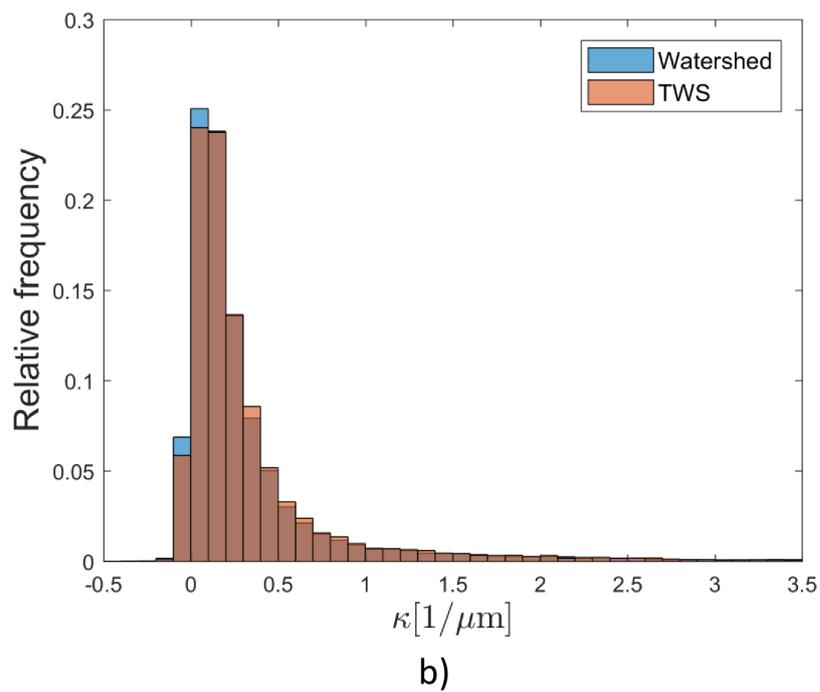
**Fig. 5** Relative frequency distributions associated with the measurements of contact angle  $\theta$  [°] and fluid-fluid interfacial mean curvature  $\kappa$  [ $1/\mu\text{m}$ ] from the same greyscale image segmented with watershed segmentation and Trainable WEKA Segmentation 3D (TWS).
