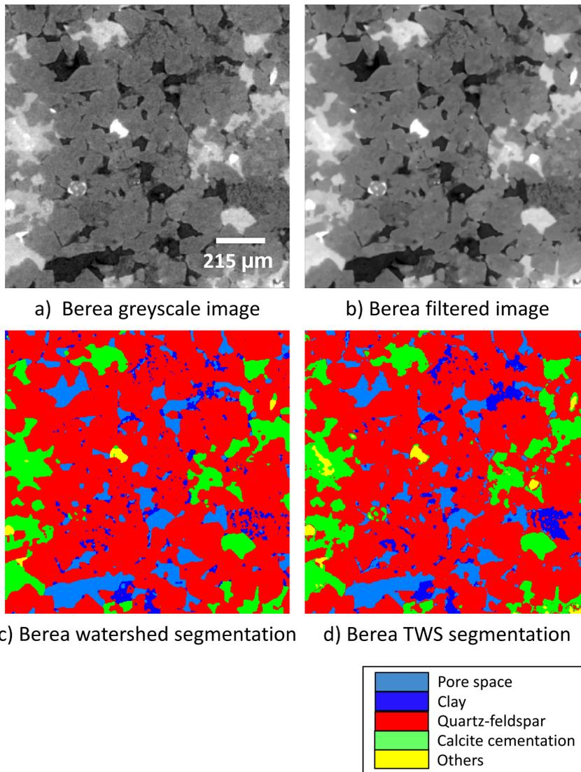
**Fig. 6** Orthogonal slices of the  $500^3$  voxels CT image of a Berea sandstone. Watershed segmentation was performed on the non-local means filtered image, while TWS was employed on the greyscale unfiltered one.
