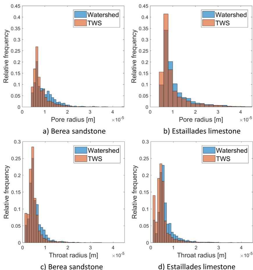
**Fig. 3** Comparison of the pore and throat radii distributions for Berea sandstone and Edwards limestone. For these samples, TWS segmentation leads to pore and throat radii distributions shifted towards smaller values. These changes explain the larger single-phase flow permeability estimates obtained from watershed segmented images.
