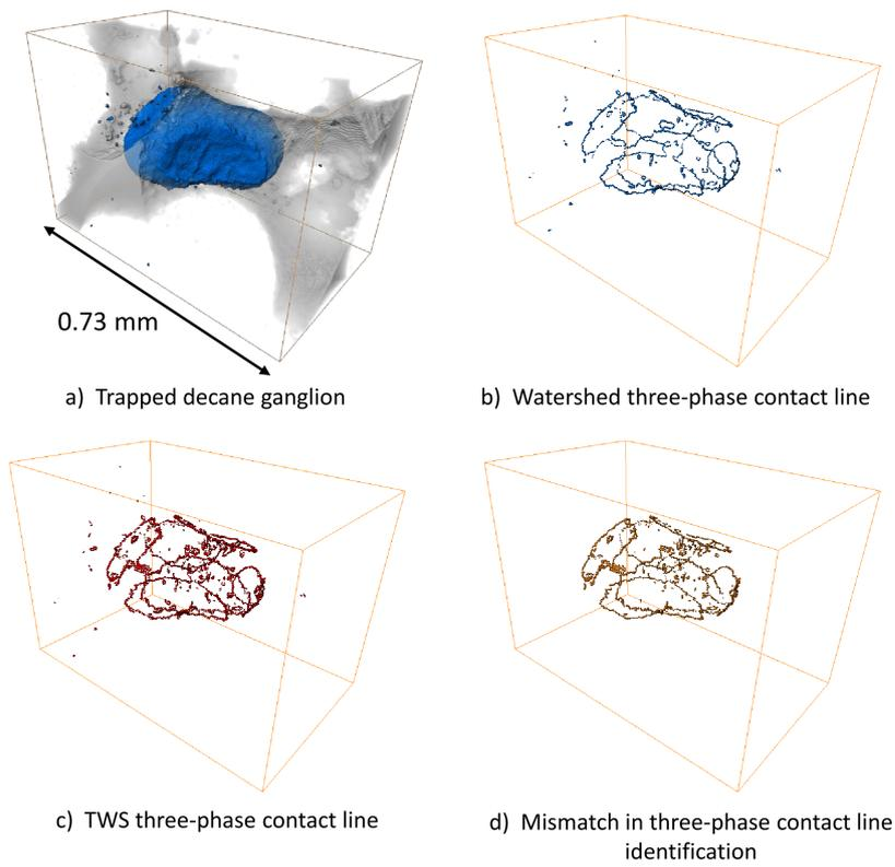
**Fig. 4** Three-phase contact lines were identified in segmented images to measure contact angles: a) Volume rendering of the segmented trapped decane ganglion; b) Contact lines identified in the image processed by non-local means filtering and watershed segmentation; c) Contact line in the image processed by Trainable WEKA Segmentation 3D (TWS); d) Differential image of the two contact lines.
