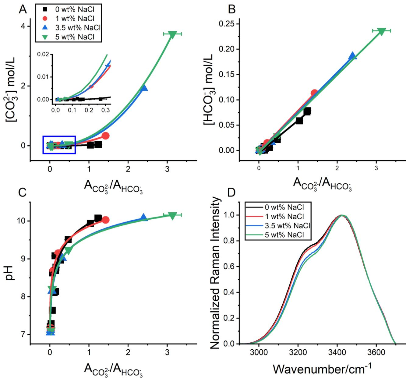
**Figure 4.** Comparisons of carbonate species concentrations ( $\text{CO}_3^{2-}$  and  $\text{HCO}_3^-$ ) and pH solution calibrations at various NaCl concentrations (salinities). Solution calibrations of  $[\text{CO}_3^{2-}]$  (A),  $[\text{HCO}_3^-]$  (B), and pH (C) versus area ratios between the  $\text{CO}_3^{2-}$  and  $\text{HCO}_3^-$  peaks. Normalized Raman  $\text{OH}^-$  stretch at different NaCl concentrations. Blue box represents the inset within (A). Concentrations are in mol/L.
