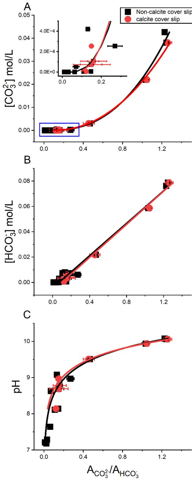
**Figure 3.** Comparisons of carbonate species concentrations and pH solution calibrations with (red) and without (black) the calcite cover slip. Solution calibrations of  $[\text{CO}_3^{2-}]$  (A),  $[\text{HCO}_3^-]$  (B), and pH (C) versus the area ratio between  $\text{CO}_3^{2-}$  and  $\text{HCO}_3^-$  peaks. Blue box represents the inset within (A). Concentrations are in mol/L.
