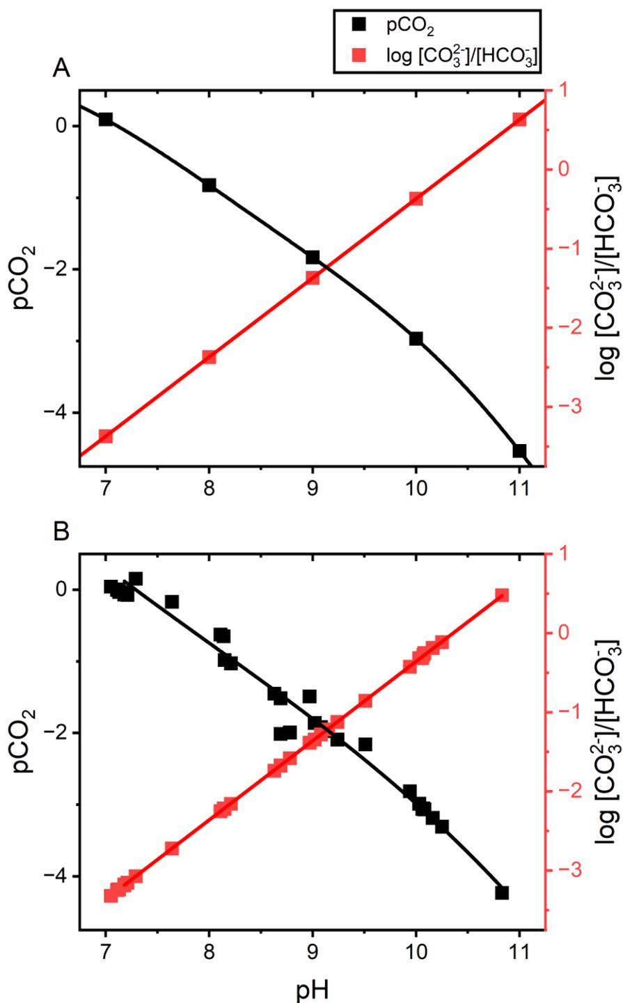
**Figure 1.** (A) Theoretical calculations of the relationship between the ratio of [CO<sub>3</sub><sup>2-</sup>] and [HCO<sub>3</sub><sup>-</sup>], pH, and pCO<sub>2</sub>. The theoretical relationship can be used to estimate pCO<sub>2</sub> over a wide range of alkaline solutions. (B) Solutions used in this study shows the relationship between the ratio of [CO<sub>3</sub><sup>2-</sup>] and [HCO<sub>3</sub><sup>-</sup>], and pH can calibrate for a wide range of pCO<sub>2</sub>.
