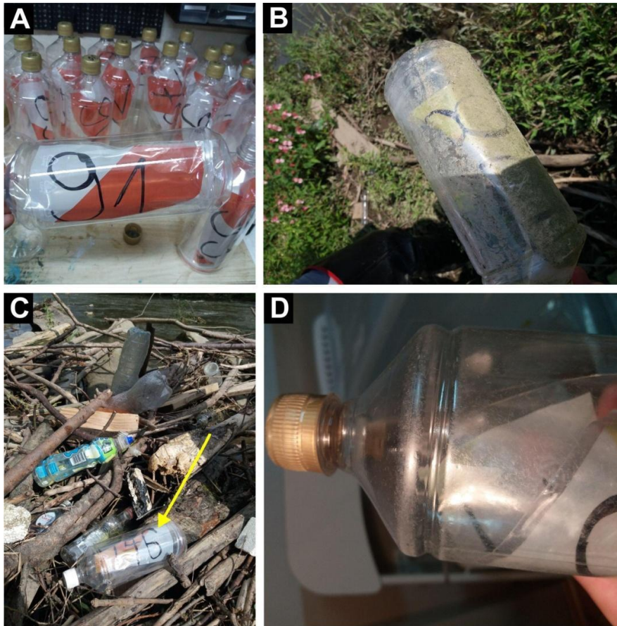
Figure 3. Tagged 1-litre PET bottles used in the experiment. Tagged bottles before (A), during (B, C) and after experiment (D). Last photo (D) indicates small cracks formed on the bottle surface during 52 days of transport in the river channel.
