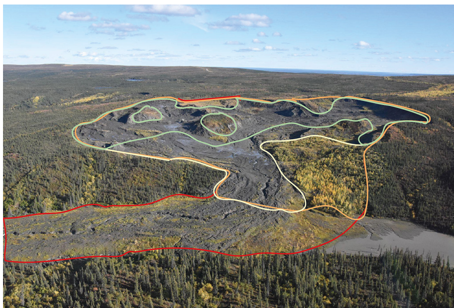
FIGURE 1 | Oblique aerial image of a typical bowl-shaped retrogressive thaw slump (RTS) in NW Canada (67.2588°, –135.2453°). Typical labeling strategies indicated: (1) only highly active regions close to the headwall in green, (2) active areas with wet bare soils including headwall and scar zone in light yellow, (3) RTS scar zone including inactive and vegetated parts in orange, and (4) complete RTS including debris tongue in red. Photo: J. Van der Sluijs. [Colour figure can be viewed at wileyonlinelibrary.com ]
