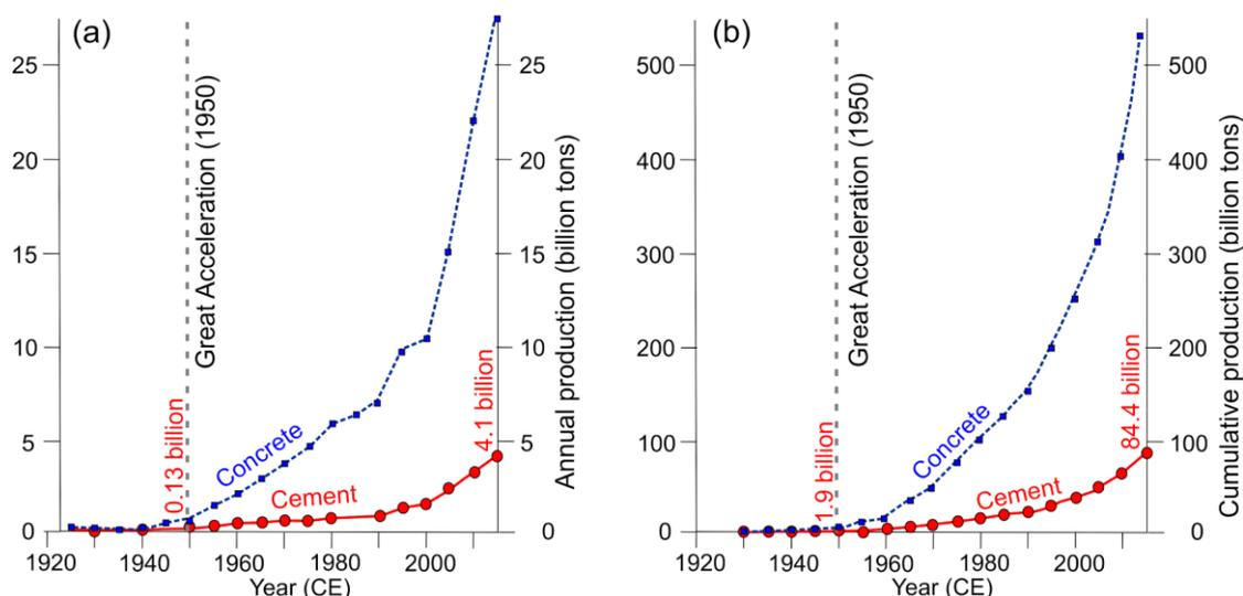
Figure 7. (a) annual global production and (b) cumulative production of cement and estimated concrete production (from Waters & Zalasiewicz, 2018).
