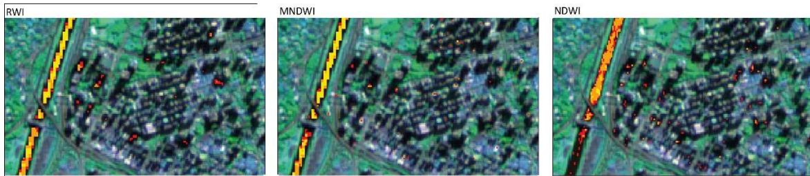
Fig. 5. Pixels classified as water, considering zero, 20, and 50 sample points as false alarms, are shown in yellow, orange, and red, respectively. Centroid coordinates -46.68683 W, -23.59242 S.
