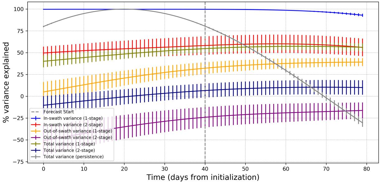
363 FIG. 8. Fraction of SSHA variance explained in one-stage and two-stage approaches, as a function of time,
